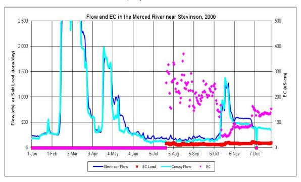
Figure F.2-3d. Daily Measured Flow (cfs) and EC ( $\mu$ S/cm) and Calculated Salt Load (tons/day) in the Merced River near Stevinson during 2000
