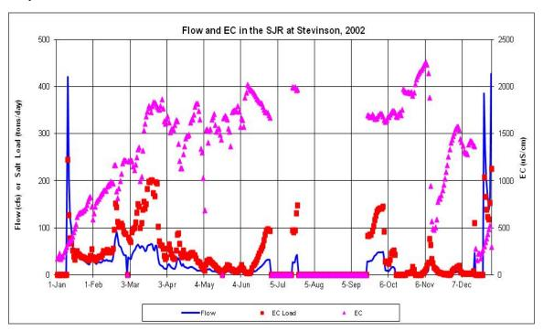
Figure F.2-5a. Daily Measured Flow (cfs) and EC ( $\mu$ S/cm) and Calculated Salt Load (tons/day) in the SJR at Stevinson during 2002
