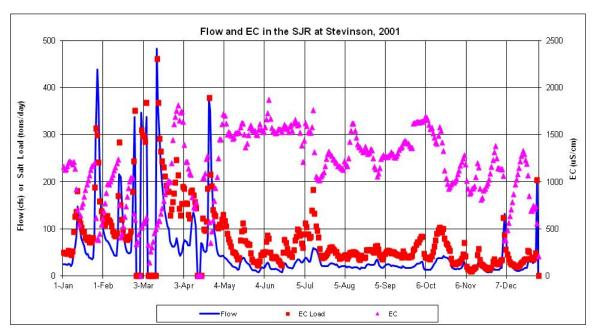
Figure F.2-4a. Daily Measured Flow (cfs) and EC ( $\mu$ S/cm) and Calculated Salt Load (tons/day) in the SJR at Stevinson during 2001
