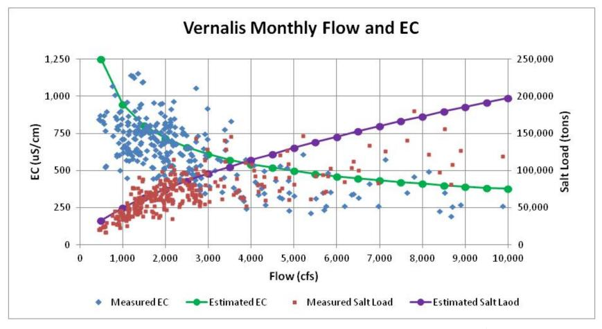
Figure F.2-1h. Relationship between SJR at Vernalis Monthly Measured Flow and EC and Calculated Salt Load for WY 1985–2011
