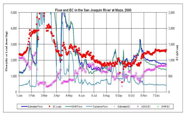
Figure F.2-3f. Daily Measured Flow (cfs) and EC ( $\mu$ S/cm) and Calculated Salt Load (tons/day) in the SJR at Maze (downstream of the Tuolumne River) during 2000
