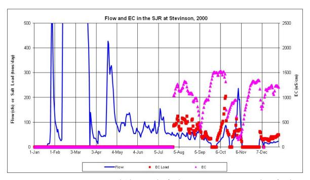
Figure F.2-3a. Daily Measured Flow (cfs) and EC ( $\mu$ S/cm) and Calculated Salt Load (tons/day) in the SJR at Stevinson during 2000
