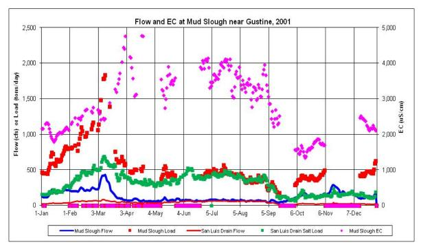
Figure F.2-4c. Daily Measured Flow (cfs) and EC ( $\mu$ S/cm) and Calculated Salt Load (tons/day) in Mud Slough near Gustine and in the San Luis Drain Discharge to Mud Slough during 2001
