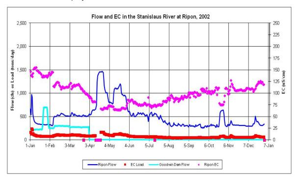
Figure F.2-5g. Daily Measured Flow (cfs) and EC ( $\mu$ S/cm) and Calculated Salt Load (tons/day) in the Stanislaus River at Ripon during 2002
