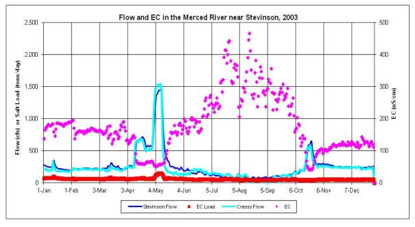
Figure F.2-6d. Daily Measured Flow (cfs) and EC ( $\mu$ S/cm) and Calculated Salt Load (tons/day) in the Merced River near Stevinson during 2003
