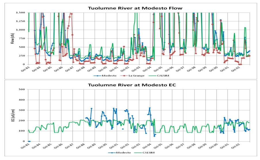
Figure F.2-2e. Comparison of CALSIM Flow and EC to the Historical Flow and EC in the Tuolumne River for WY 1985–2003
