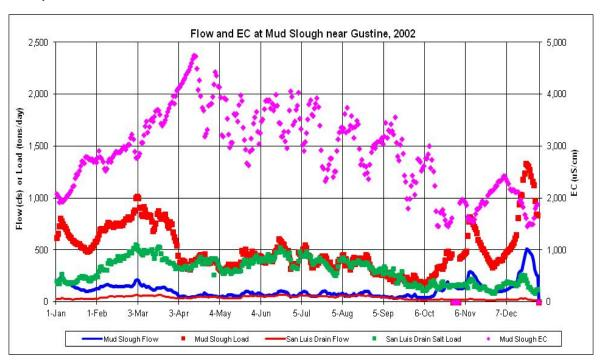
Figure F.2-5c. Daily Measured Flow (cfs) and EC ( $\mu$ S/cm) and Calculated Salt Load (tons/day) in Mud Slough near Gustine and in the San Luis Drain Discharge to Mud Slough during 2002
