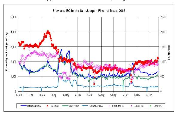
Figure F.2-6f. Daily Measured Flow (cfs) and EC ( $\mu$ S/cm) and Calculated Salt Load (tons/day) in the SJR at Maze (downstream of the Tuolumne River) during 2003
