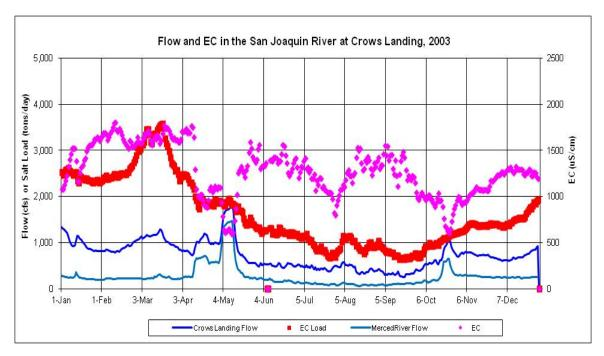
Figure F.2-6e. Daily Measured Flow (cfs) and EC ( $\mu$ S/cm) and Calculated Salt Load (tons/day) in the SJR at Crows Landing (downstream of the Merced River) during 2003
