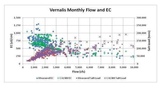
Figure F.2-2i. Comparison of CALSIM Flow, EC and Salt Load to the Historical Flow, EC and Salt Load in the San Joaquin River at Vernalis for WY 1985–2003
