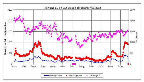
Figure F.2-5b. Daily Measured Flow (cfs) and EC ( $\mu$ S/cm) and Calculated Salt Load (tons/day) in Salt Slough at Highway 165 during 2002
