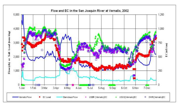
Figure F.2-5h. Daily Measured Flow (cfs) and EC ( $\mu$ S/cm) and Calculated Salt Load (tons/day) in the San Joaquin River at Vernalis during 2002
