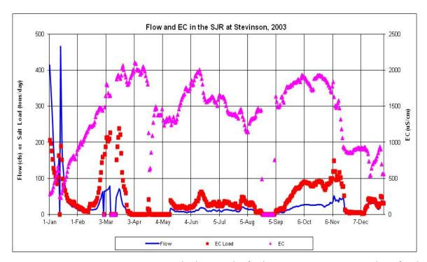
Figure F.2-6a. Daily Measured Flow (cfs) and EC ( $\mu$ S/cm) and Calculated Salt Load (tons/day) in the SJR at Stevinson during 2003
