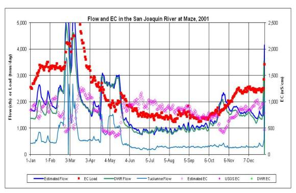
Figure F.2-4f. Daily Measured Flow (cfs) and EC ( $\mu$ S/cm) and Calculated Salt Load (tons/day) in the SJR at Maze (downstream of the Tuolumne River) during 2001
