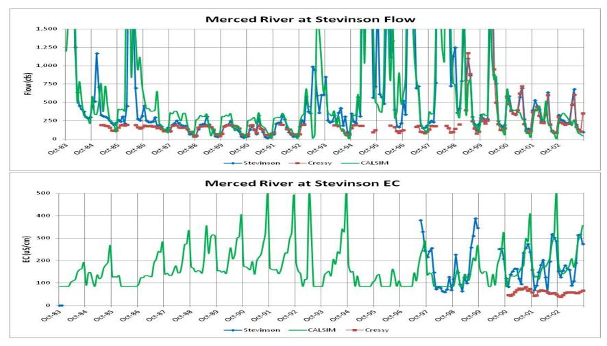
Figure F.2-2b. Comparison of CALSIM Flow and EC to the Historical Flow and EC in the Merced River for WY 1985-2003
