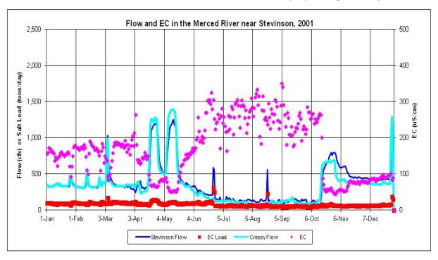
Figure F.2-4d. Daily Measured Flow (cfs) and EC ( $\mu$ S/cm) and Calculated Salt Load (tons/day) in the Merced River near Stevinson during 2001
