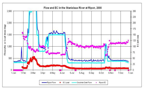
Figure F.2-3g. Daily Measured Flow (cfs) and EC ( $\mu$ S/cm) and Calculated Salt Load (tons/day) in the Stanislaus River at Ripon during 2000
