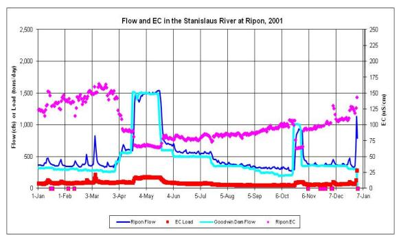
Figure F.2-4g. Daily Measured Flow (cfs) and EC ( $\mu$ S/cm) and Calculated Salt Load (tons/day) in the Stanislaus River at Ripon during 2001
