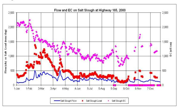
Figure F.2-3b. Daily Measured Flow (cfs) and EC ( $\mu$ S/cm) and Calculated Salt Load (tons/day) in Salt Slough at Highway 165 during 2000
