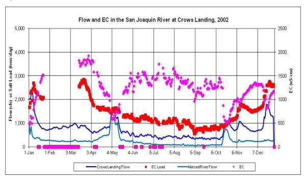
Figure F.2-5e. Daily Measured Flow (cfs) and EC ( $\mu$ S/cm) and Calculated Salt Load (tons/day) in the SJR at Crows Landing (downstream of the Merced River) during 2002
