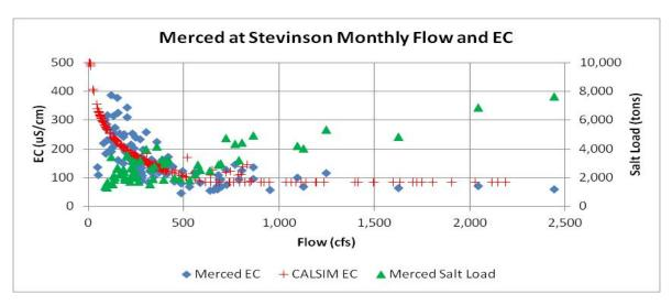
Figure F.2-2d. Comparison of CALSIM EC to the Historical Flow, EC and Salt Load in the Merced River for WY 1985–2003
