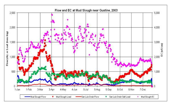
Figure F.2-6c. Daily Measured Flow (cfs) and EC ( $\mu$ S/cm) and Calculated Salt Load (tons/day) in Mud Slough near Gustine and in the San Luis Drain Discharge to Mud Slough during 2003
