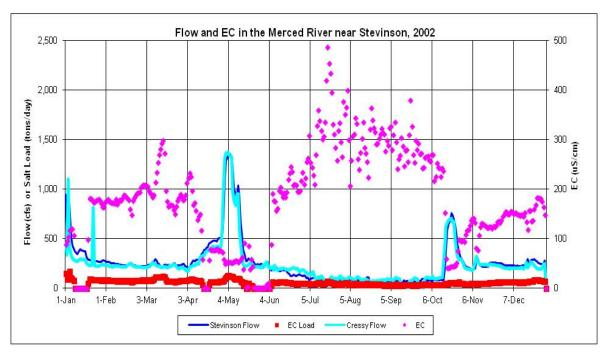
Figure F.2-5d. Daily Measured Flow (cfs) and EC ( $\mu$ S/cm) and Calculated Salt Load (tons/day) in the Merced River near Stevinson during 2002
