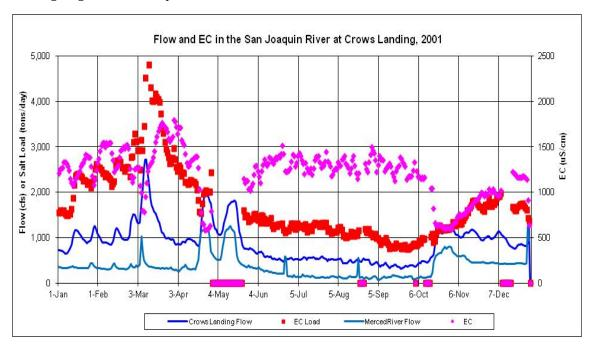
Figure F.2-4e. Daily Measured Flow (cfs) and EC ( $\mu$ S/cm) and Calculated Salt Load (tons/day) in the SJR at Crows Landing (downstream of the Merced River) during 2001
