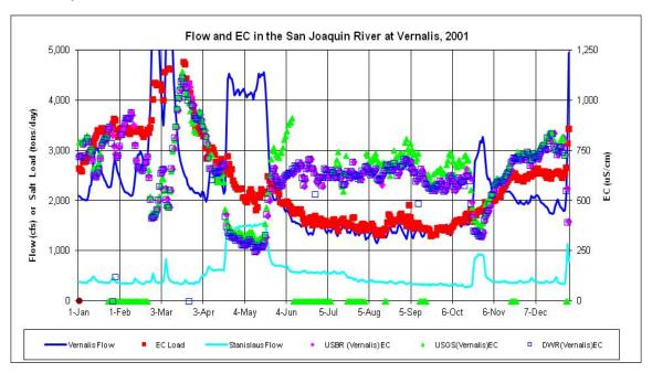
Figure F.2-4h. Daily Measured Flow (cfs) and EC ( $\mu$ S/cm) and Calculated Salt Load (tons/day) in the San Joaquin River at Vernalis during 2001
