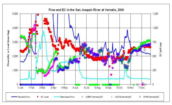
Figure F.2-3h. Daily Measured Flow (cfs) and EC ( $\mu$ S/cm) and Calculated Salt Load (tons/day) in the San Joaquin River at Vernalis during 2000
