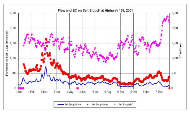
Figure F.2-4b. Daily Measured Flow (cfs) and EC ( $\mu$ S/cm) and Calculated Salt Load (tons/day) in Salt Slough at Highway 165 during 2001
