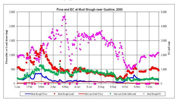
Figure F.2-3c. Daily Measured Flow (cfs) and EC ( $\mu$ S/cm) and Calculated Salt Load (tons/day) in Mud Slough near Gustine and in the San Luis Drain Discharge to Mud Slough during 2000
