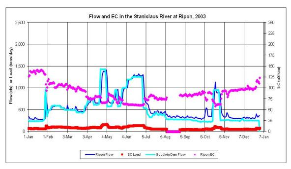
Figure F.2-6g. Daily Measured Flow (cfs) and EC ( $\mu$ S/cm) and Calculated Salt Load (tons/day) in the Stanislaus River at Ripon during 2003
