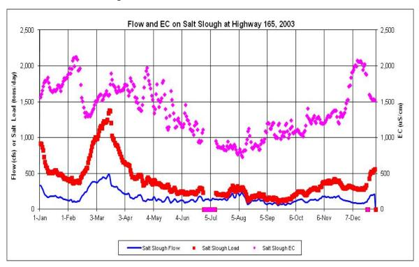
Figure F.2-6b. Daily Measured Flow (cfs) and EC ( $\mu$ S/cm) and Calculated Salt Load (tons/day) in Salt Slough at Highway 165 during 2003
