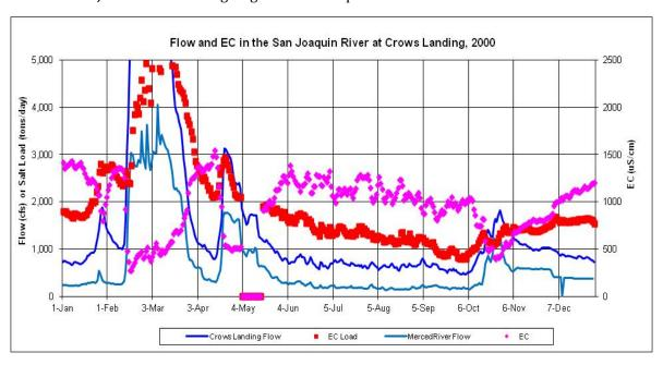
Figure F.2-3e. Daily Measured Flow (cfs) and EC ( $\mu$ S/cm) and Calculated Salt Load (tons/day) in the SJR at Crows Landing (downstream of the Merced River) during 2000
