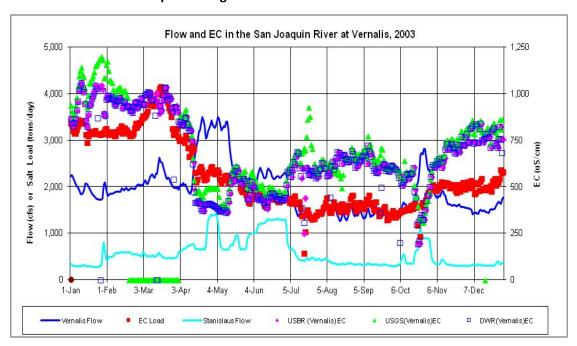
Figure F.2-6h. Daily Measured Flow (cfs) and EC ( $\mu$ S/cm) and Calculated Salt Load (tons/day) in the San Joaquin River at Vernalis during 2003
