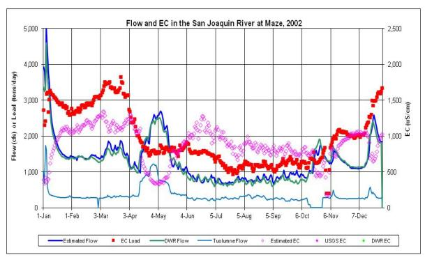
Figure F.2-5f. Daily Measured Flow (cfs) and EC ( $\mu$ S/cm) and Calculated Salt Load (tons/day) in the SJR at Maze (downstream of the Tuolumne River) during 2002
