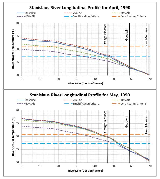
Figure F.1.6-23. Longitudinal Monthly Average 7DADM Temperature Results within the Stanislaus River for (a) April 1990 and (b) May 1990
