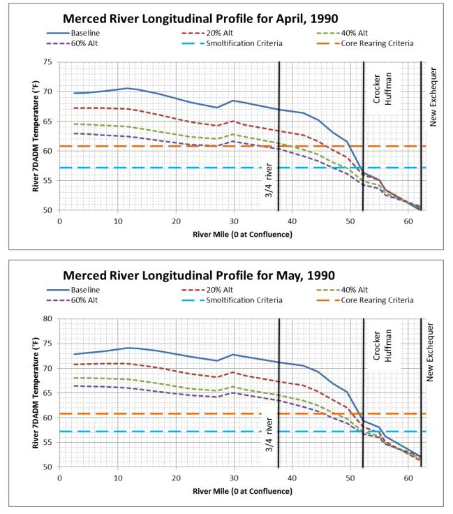
Figure F.1.6-59. Longitudinal Monthly Average 7DADM Temperature Results within the Merced River for (a) April 1990 and (b) May 1990
