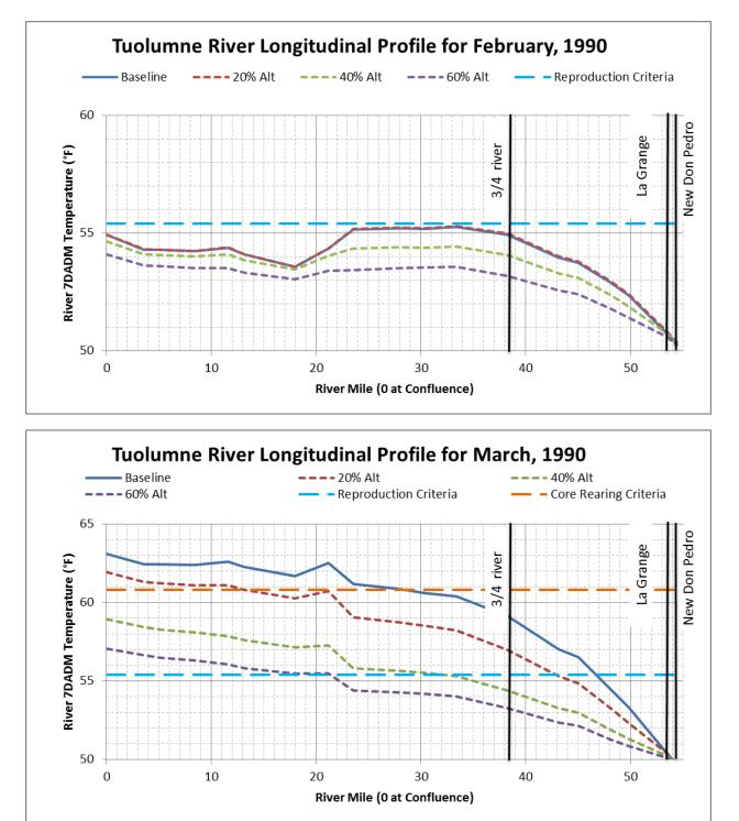
Figure F.1.6-40. Longitudinal Monthly Average 7DADM Temperature Results within the Tuolumne River for (a) February 1990 and (b) March 1990
