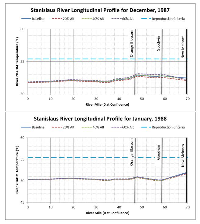
Figure F.1.6-15. Longitudinal Monthly Average 7DADM Temperature Results within the Stanislaus River for (a) December 1987 and (b) January 1988
