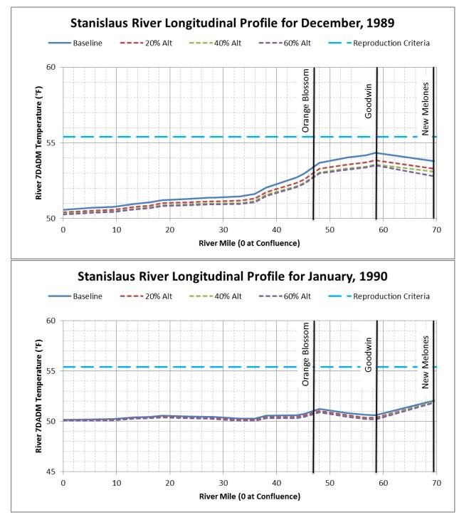
Figure F.1.6-21. Longitudinal Monthly Average 7DADM Temperature Results within the Stanislaus River for (a) December 1989 and (b) January 1990
