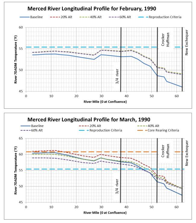
Figure F.1.6-58. Longitudinal Monthly Average 7DADM Temperature Results within the Merced River for (a) February 1990 and (b) March 1990
