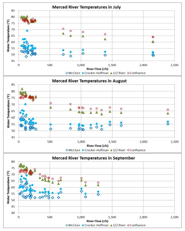
Figure F.1.6-7d. Effects of Merced River Flow on Merced River Water Temperatures July–September for Baseline Conditions 1970–2003
