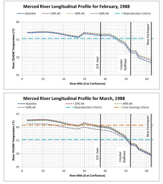
Figure F.1.6-52. Longitudinal Monthly Average 7DADM Temperature Results within the Merced River for (a) February 1988 and (b) March 1988
