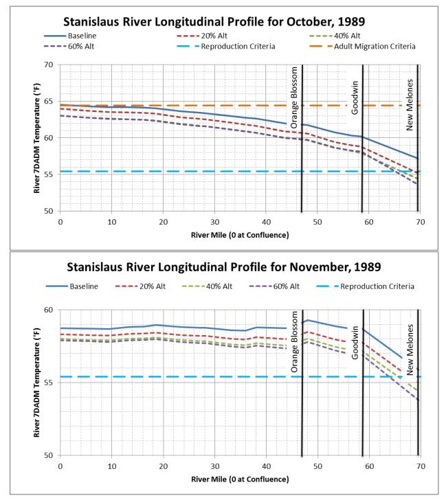
Figure F.1.6-20. Longitudinal Monthly Average 7DADM Temperature Results within the Stanislaus River for (a) October 1989 and (b) November 1989
