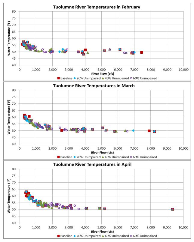
Figure F.1.6-26a. Effects of Tuolumne River Flows on Temperatures at RM 28.1 in February–April for Baseline Conditions and 20%, 40%, 60% Unimpaired Flow (LSJR Alternatives 2–4) 1970–2003
