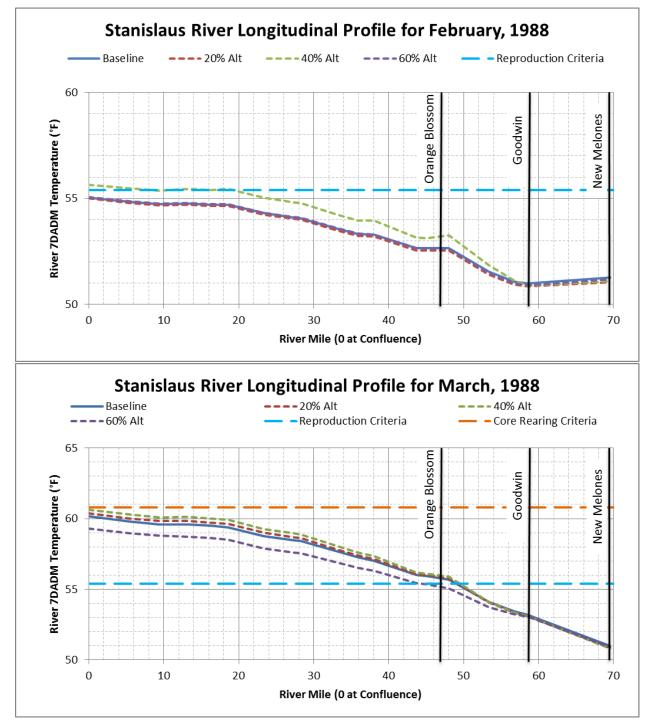
Figure F.1.6-16. Longitudinal Monthly Average 7DADM Temperature Results within the Stanislaus River for (a) February 1988 and (b) March 1988
