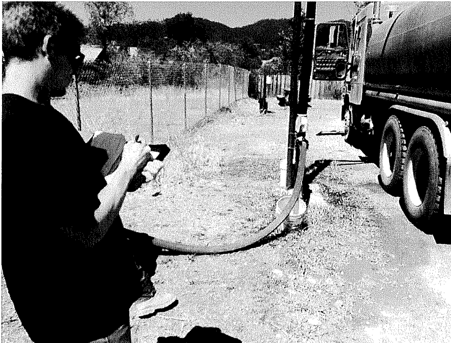
Photo 2 – 3,800 gallon water truck filling up.
