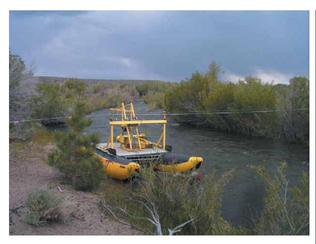
Figure 24b. Cataraft set-up at the Lower Rush Creek site, June 25, 2005. Bank configuration on the left channel margin and vegetation along the right channel margin prevented the reel-operated samplers (TR-2 and D-74) to be used along the edges, so sampling along both channel edges was performed with hand-held samplers (3-inch Helley-Smith and DH-48). View is from the left bank, flow is from lower right and is approximately 465 cfs.
