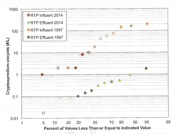
Figure 4-1 RTP Cryptosporidium oocyst distributions (open circles indicate the concentration was below the plotted value)
