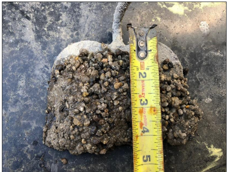
Photograph 2.1 – Gravel removed from the bottom of well using Mud Rotary Rig before destruction. Photograph taken on June 24, 2020.
