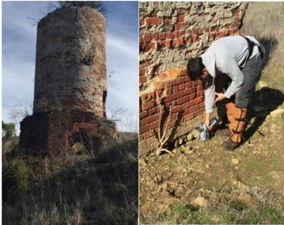
Figure 3. Ore roasting furnace and mercury analysis with X-Ray Fluorescence Spectrometer by Nicholas Piucci.
