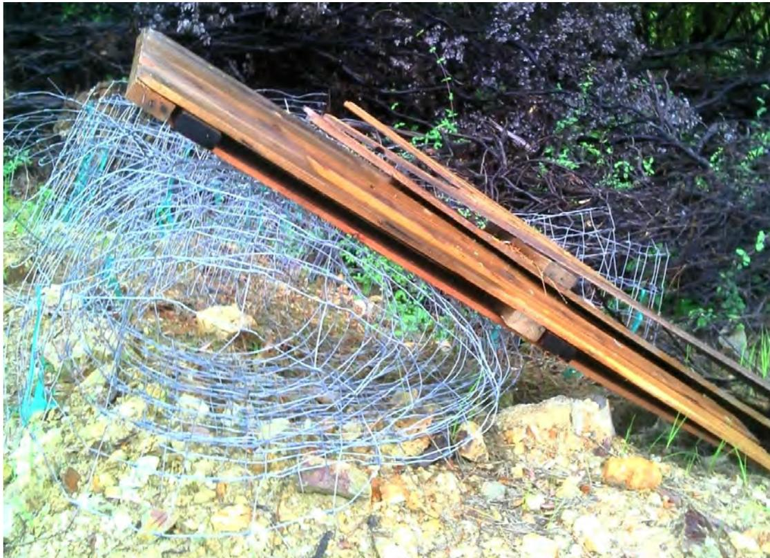
Photo 49-50: Severely weathered sediment control waddles.
