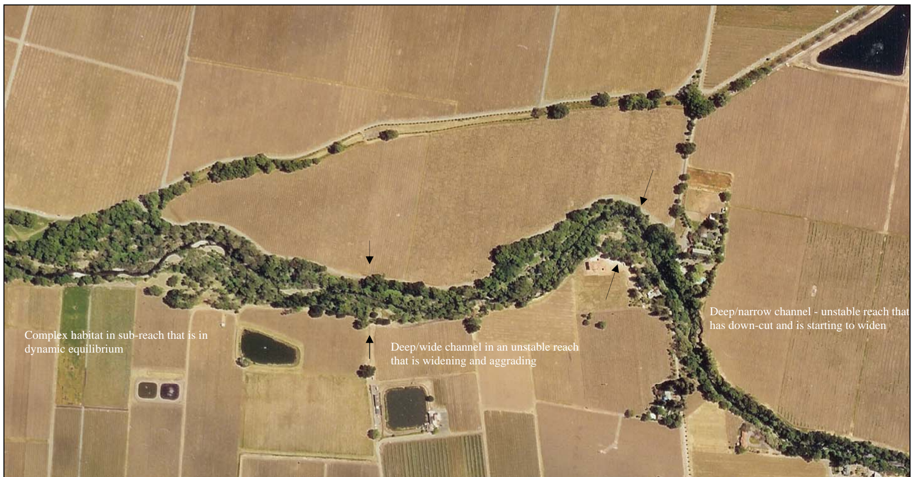
Figure 12: Aerial photograph of the Rutherford Reach of the Napa River showing the channel from about 2000-7500 ft. downstream of Rutherford Cross Road. This aerial photo was taken in 2002. Direction of flow is from left to right. Upstream of the first set of arrows, the channel is much wider and shallower and habitat is much more complex than elsewhere in the photo, and characterized by gravel bars and riffles (light colored arcs) that with pools. Between the two sets of arrows, the channel is deeper, somewhat narrower, and habitat is less complex than immediately upstream, and here the channel is actively widening and filling in. In contrast to other areas shown in the photograph, downstream of the second set of arrows, the channel is much narrower and less complex, and pools and deep-runs are dominant habitats.
