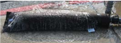
Water pumping through the C.I.Agent® EVAC Filter while it catches and contains hydrocarbons.
