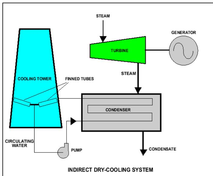
Figure 4-7. Indirect Dry Cooling
