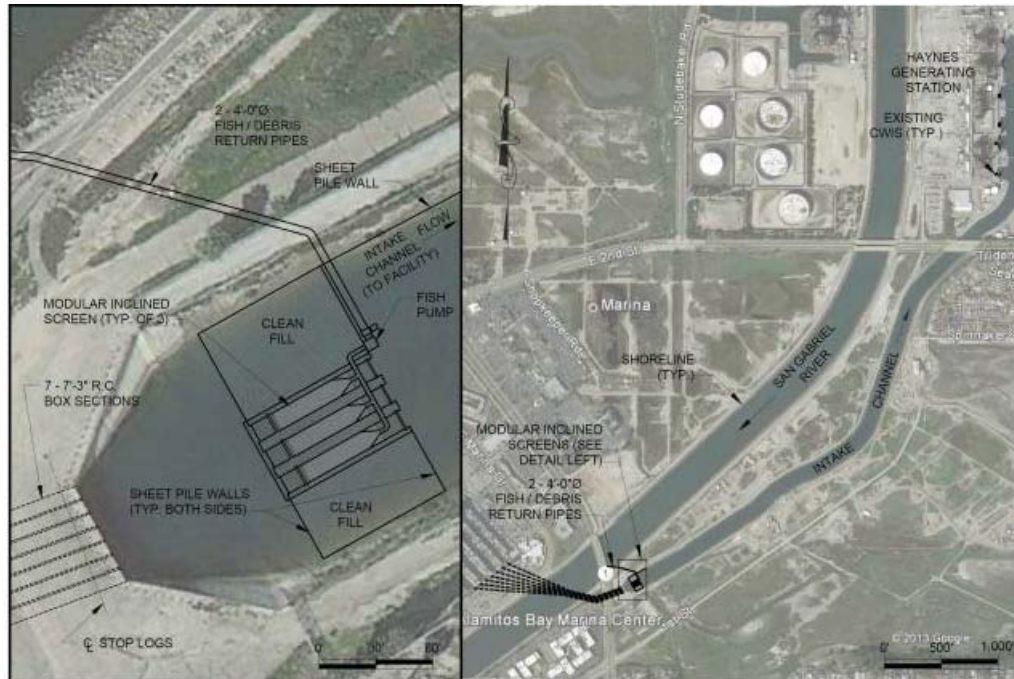
Figure 4.2 – Modular inclined screens at Haynes
