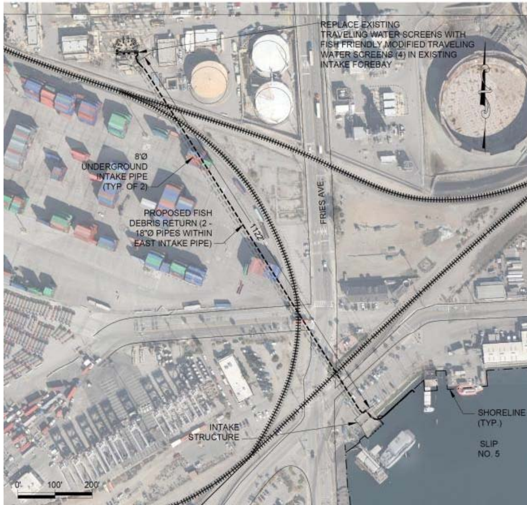
Figure 3.1 – Fish-friendly modified traveling water screen retrofit option for Harbor
