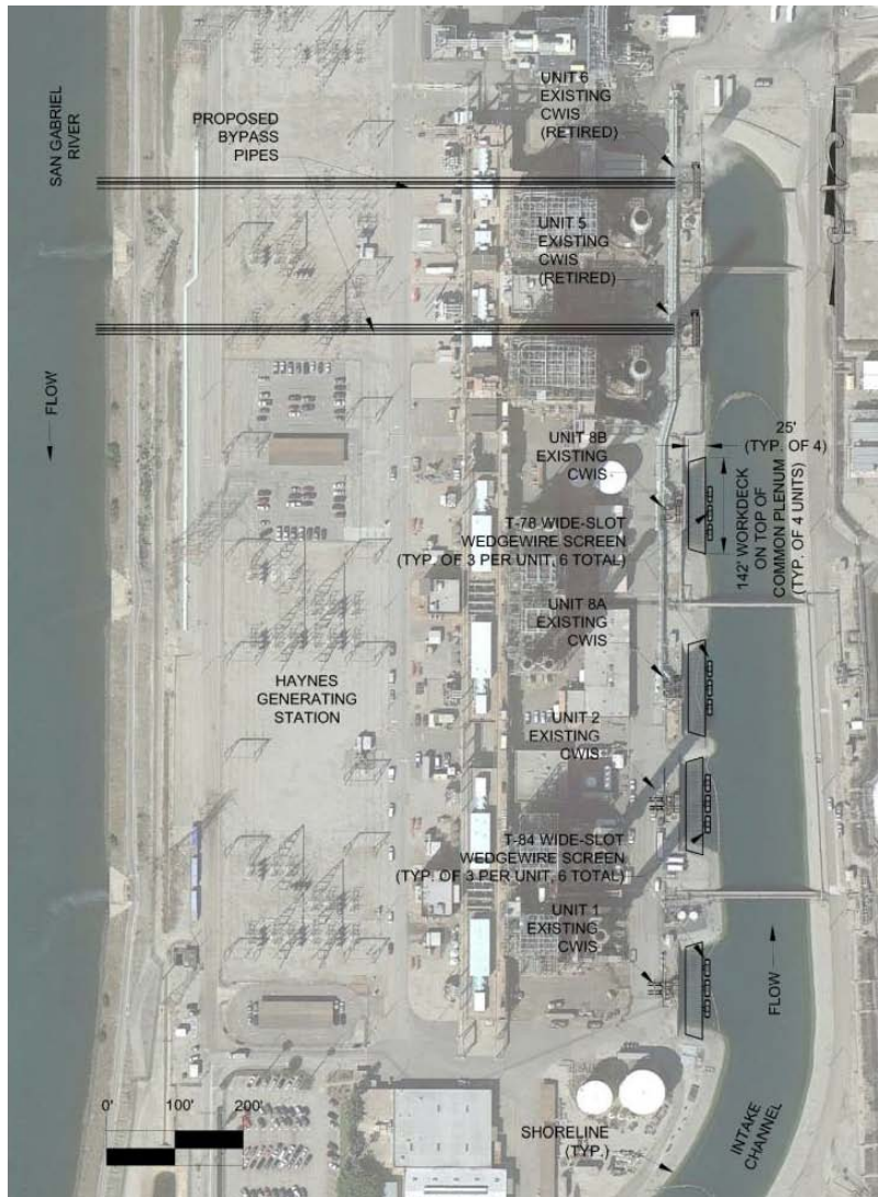
Figure 4.3 – Wide-slot wedgewire Screens at Haynes
