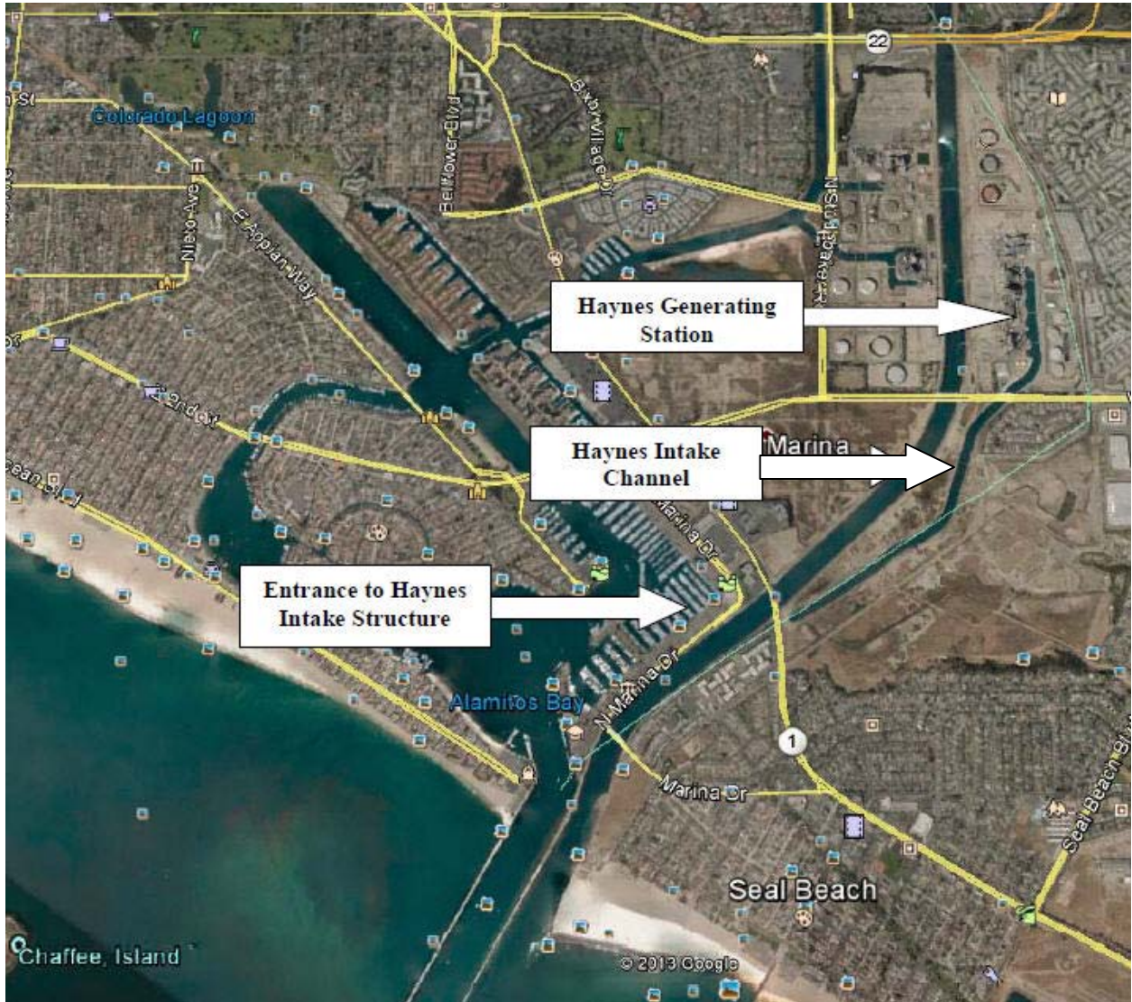
Figure 1.3 – Location of the Haynes Generating Station intake channel and entrance to the cooling water intake structure.
