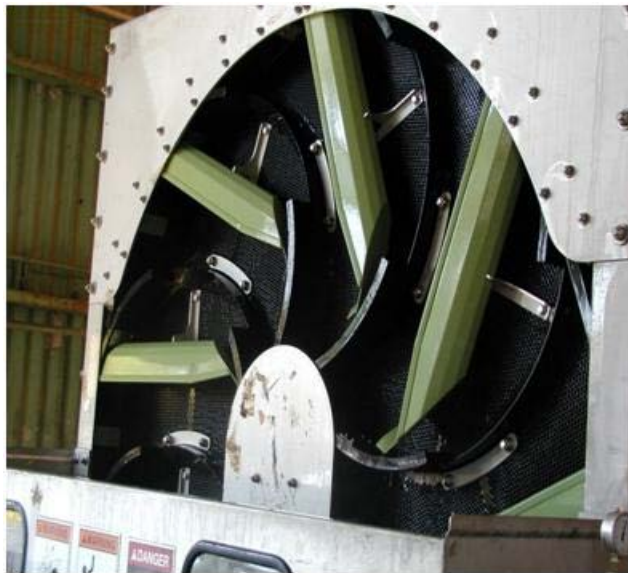
Figure A-4 Passavant-Geiger Multi-Disc Screen (Courtesy of Passavant-Geiger).
