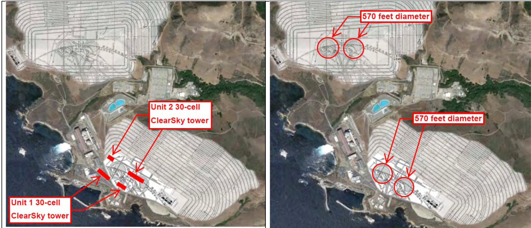
Figure D. 30-cell ClearSky™ Southern Location (with No Excavation Necessary) Compared to Round Towers Evaluated by Bechtel with Extensive Excavation
