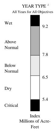
A cap of 10.0 MAF is put on the previous year's index (Z) to account for required flood control reservoir releases during wet years.
