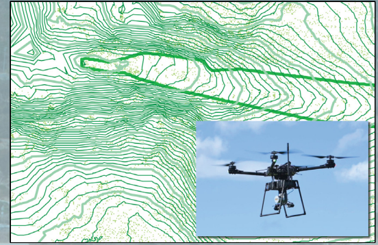
IR 7 ravine topography captured via LiDAR-equipped drone (inset)
