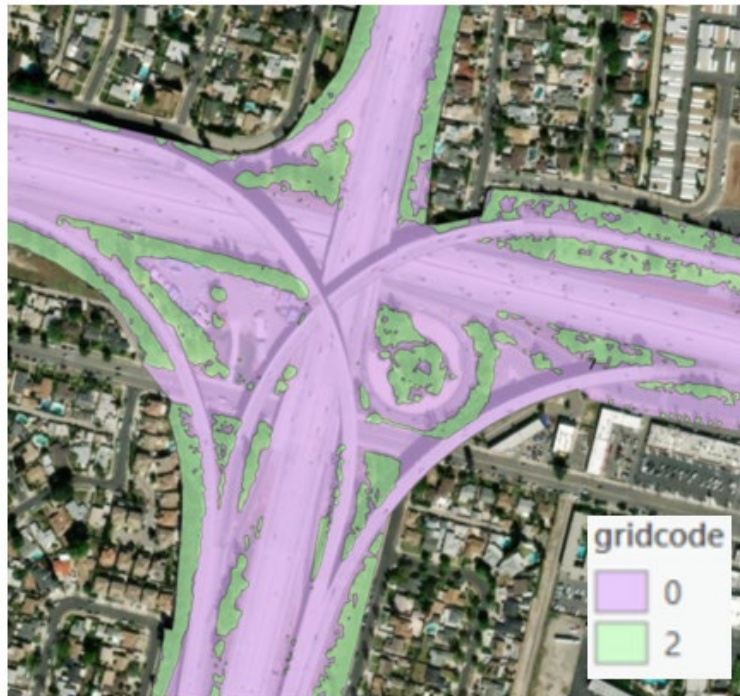
Figure 1: Final Landcover Classification Polygons (gridcode 0 = non-vegetated, gridcode 2 = vegetated)
