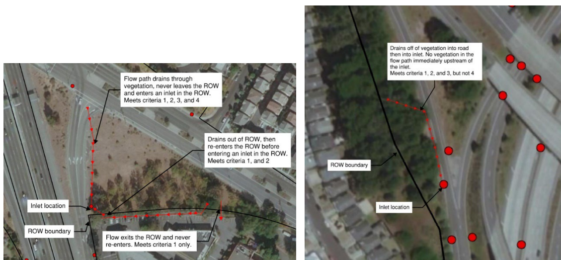
Figure 5: Visualization of example criteria described in section 4.4.
