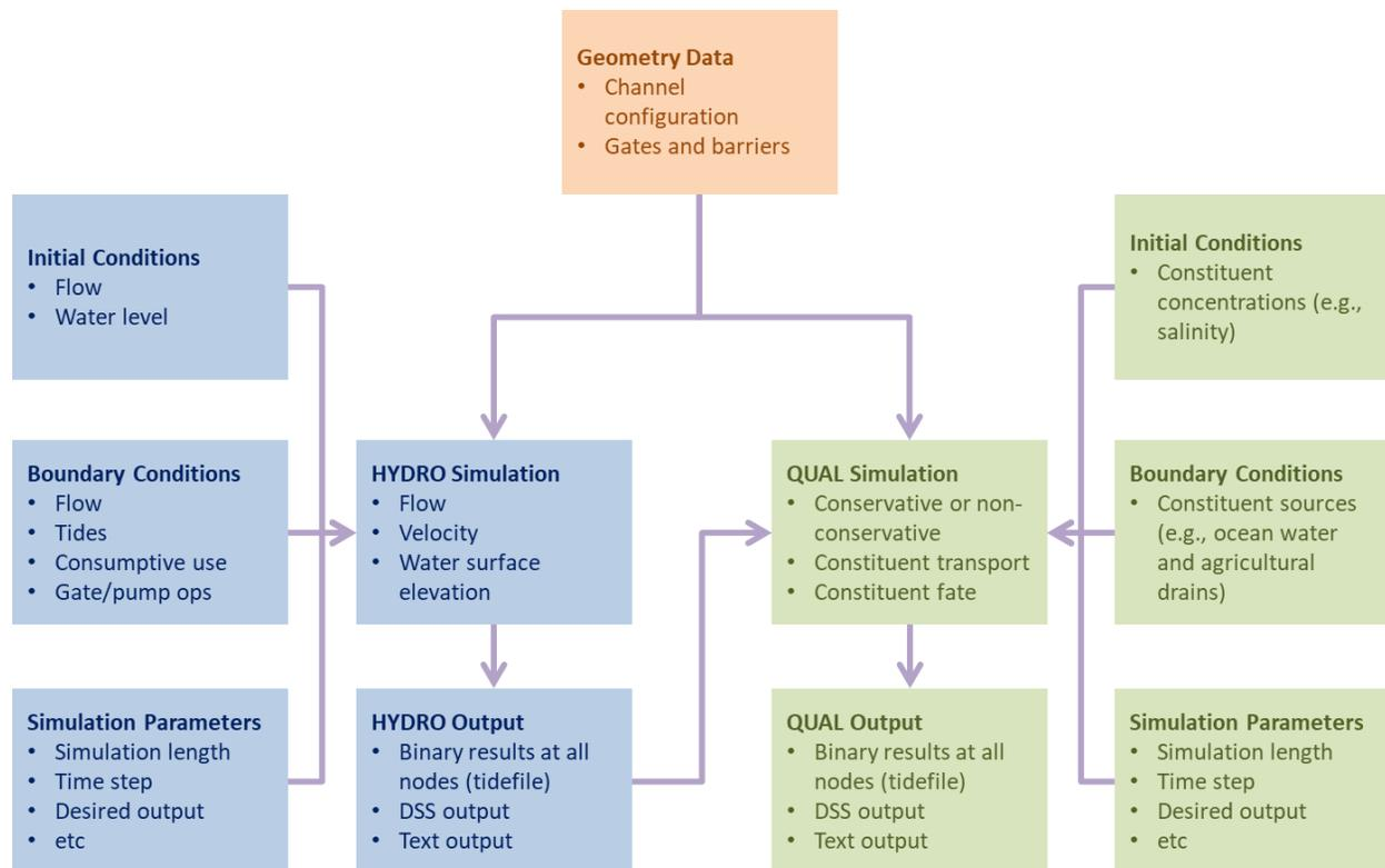
**Figure 3. Flow Chart of HYDRO and QUAL Inputs and Outputs**
