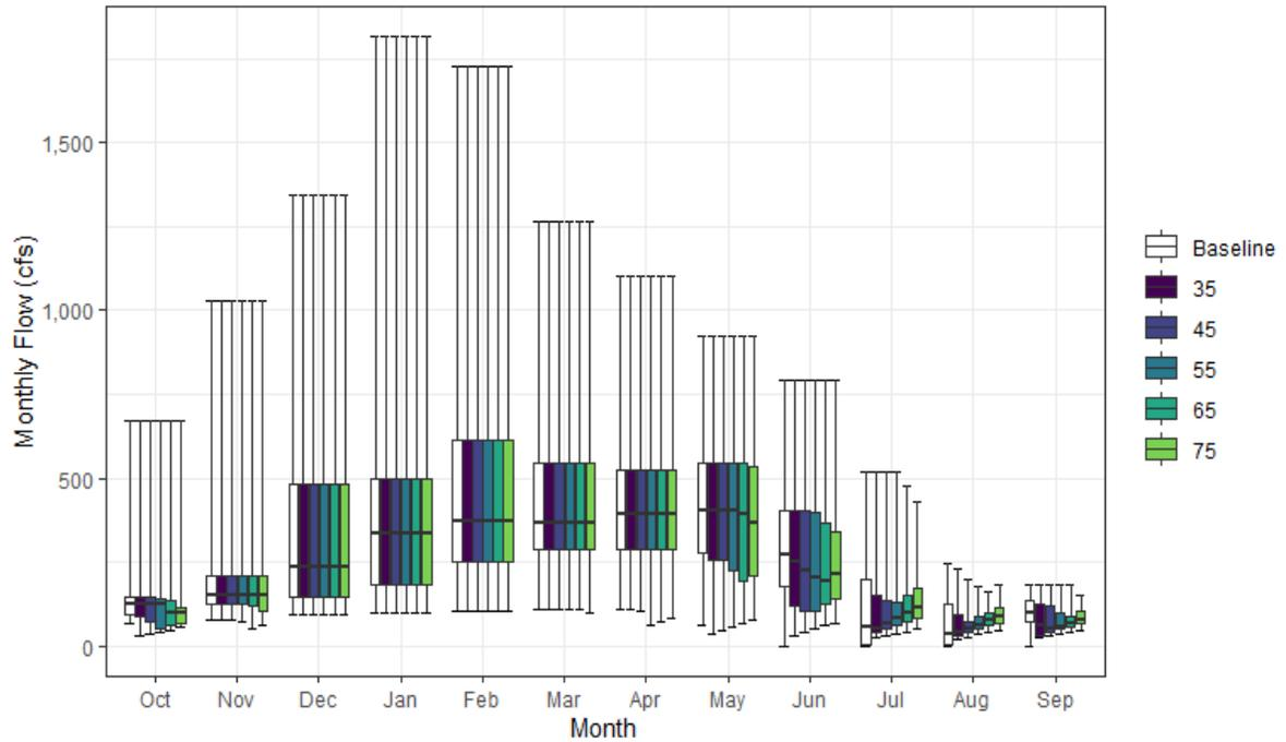
Changes represent the typical patterns for unregulated tributaries with high surface water demand. Modeled reductions in flow result from limitations in the spatial resolution of agricultural demands in SacWAM. cfs = cubic feet per second
