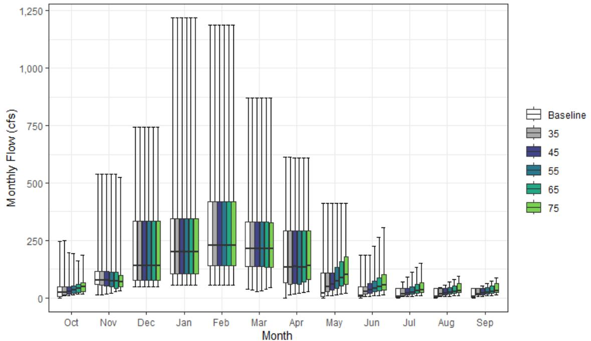
Changes represent the typical patterns for unregulated tributaries with high surface water demand. cfs = cubic feet per second
