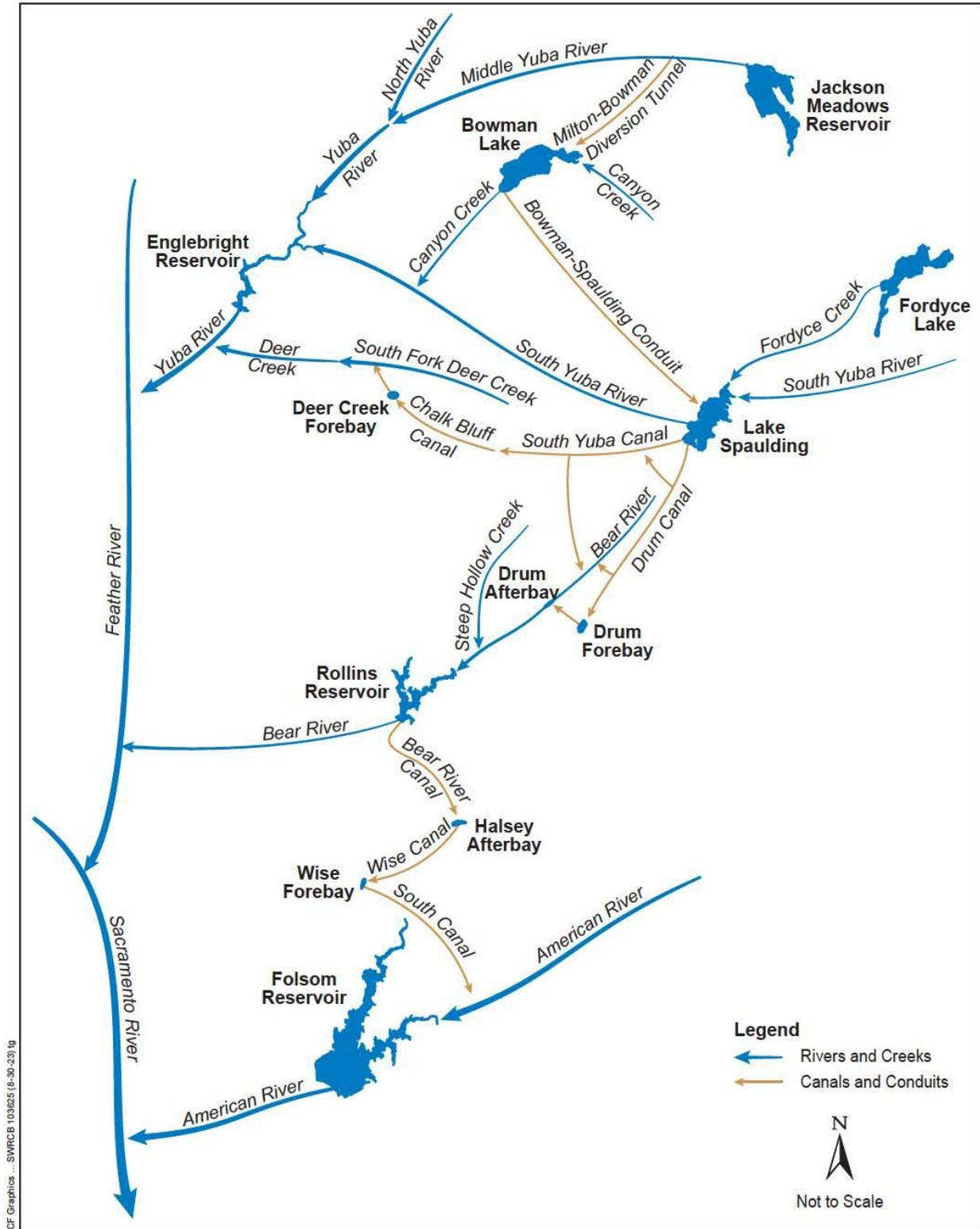
Figure 6.3-23. Example of an Interbasin Diversion (Yuba-Bear Project)
