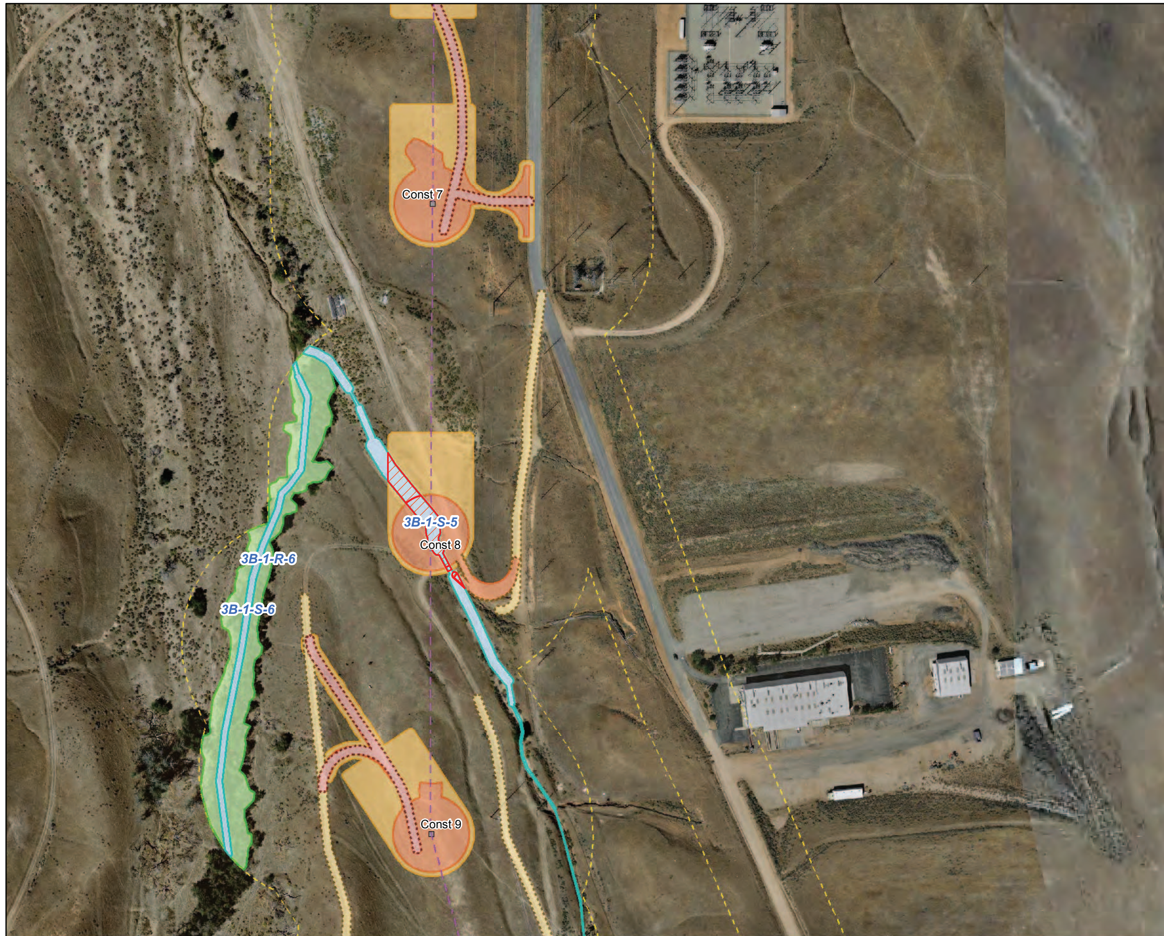
Figure 5 Representative Map of Impacts to Waters under the Water Board and CDFG Jurisdictions (Construct 8 – permanent tower footing O&M area in drainage) Attachment D Antelope Transmission Project – Segment 3B
