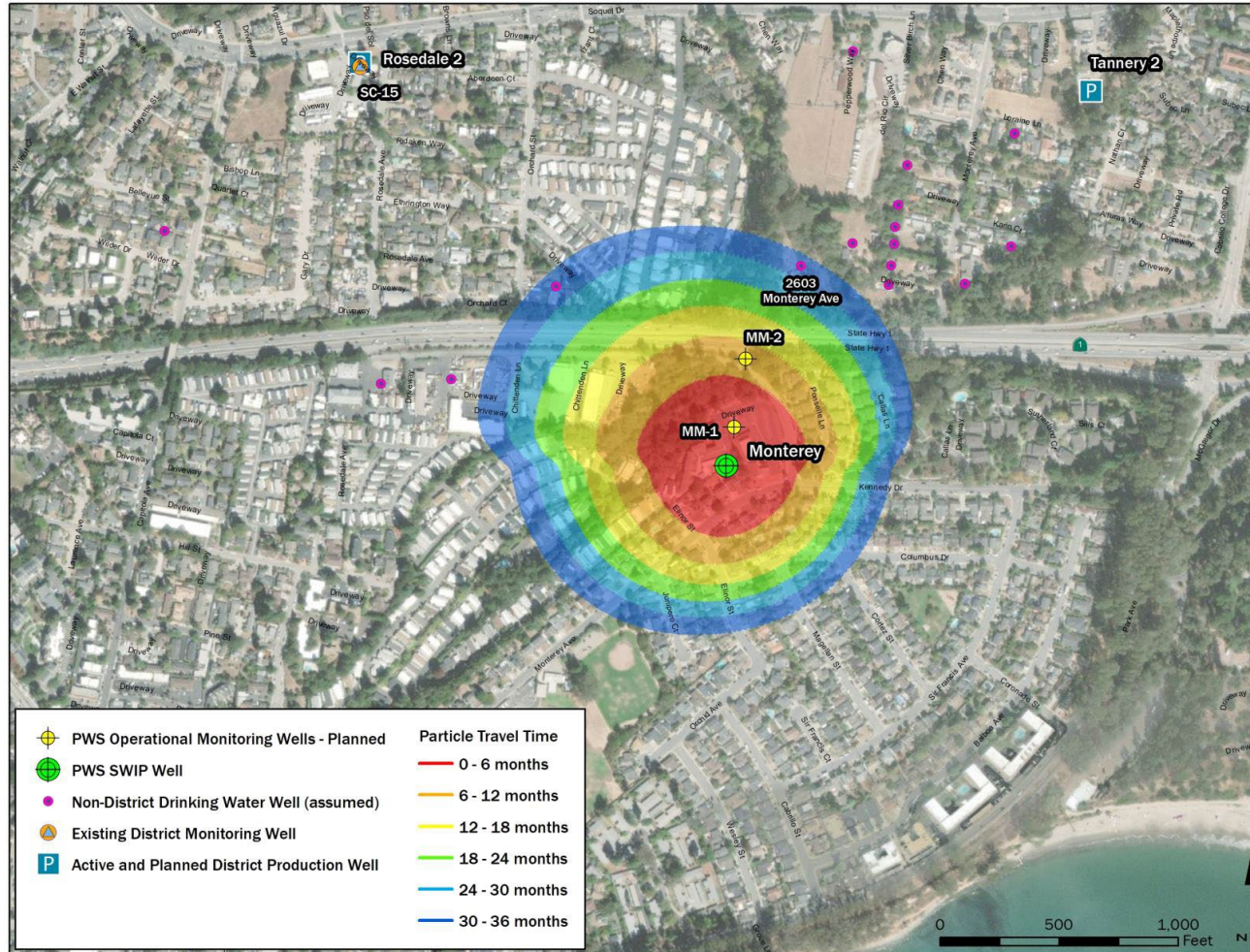
Figure C-3. Map of Monterey SWIP well, two monitoring wells (MM-1 and MM-2), and modeled subsurface travel times in Purisima A Unit from the SWIP well. PWS denotes Pure Water Soquel. Figure is from the Final Pure Water Soquel Engineering Report prepared for Soquel Creek Water District, March 2023.
