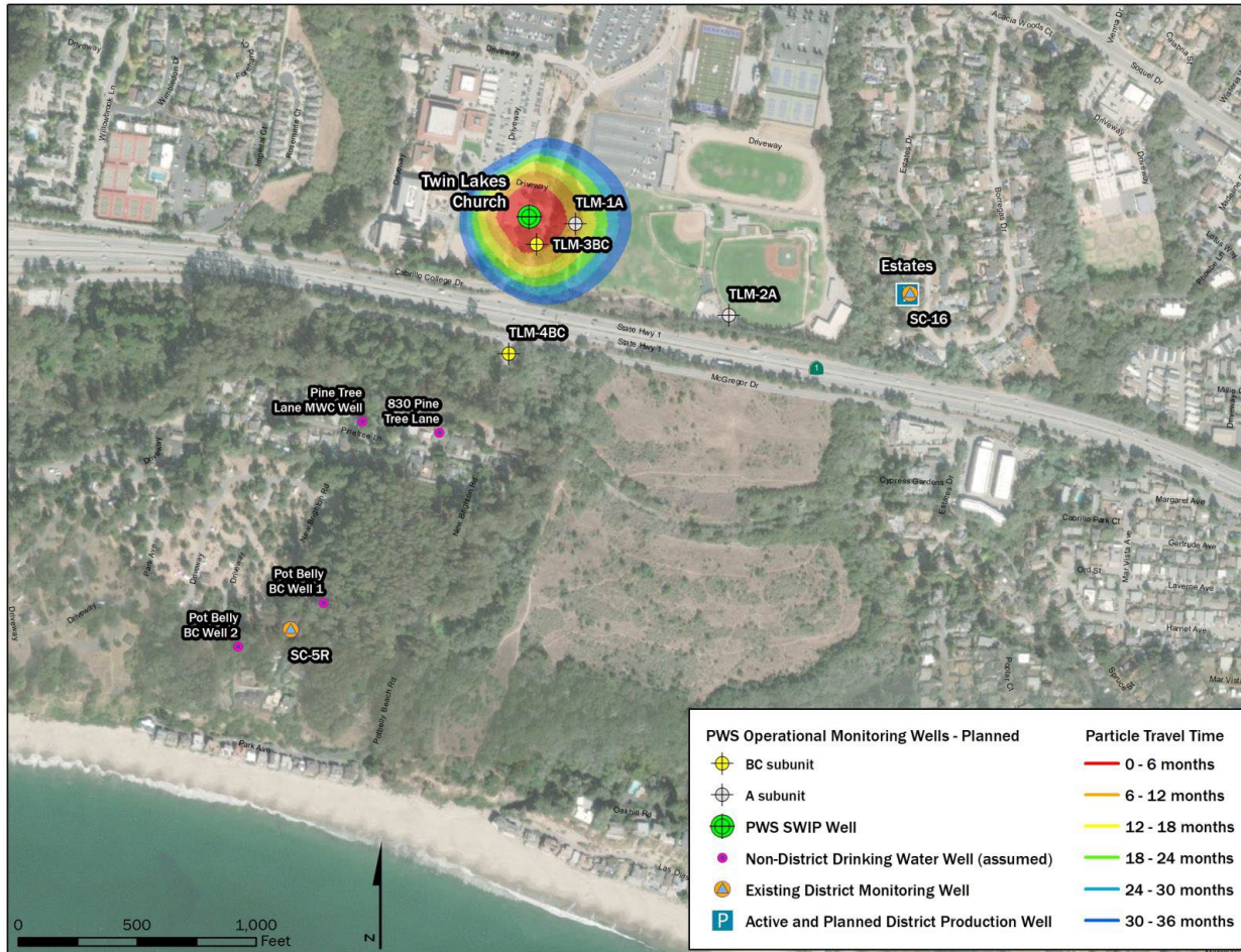
Figure C-6. Map of Twin Lakes Church (TLC) SWIP well, monitoring wells for the Purisima Unit A (TLM-1A and TLM-2A) and Purisima Unit BC (TLM-3BC and TLM-4BC), and modeled subsurface travel times in the Purisima B Unit from the SWIP well. Figure is from the Final Pure Water Soquel Engineering Report prepared for Soquel Creek Water District, March 2023.
