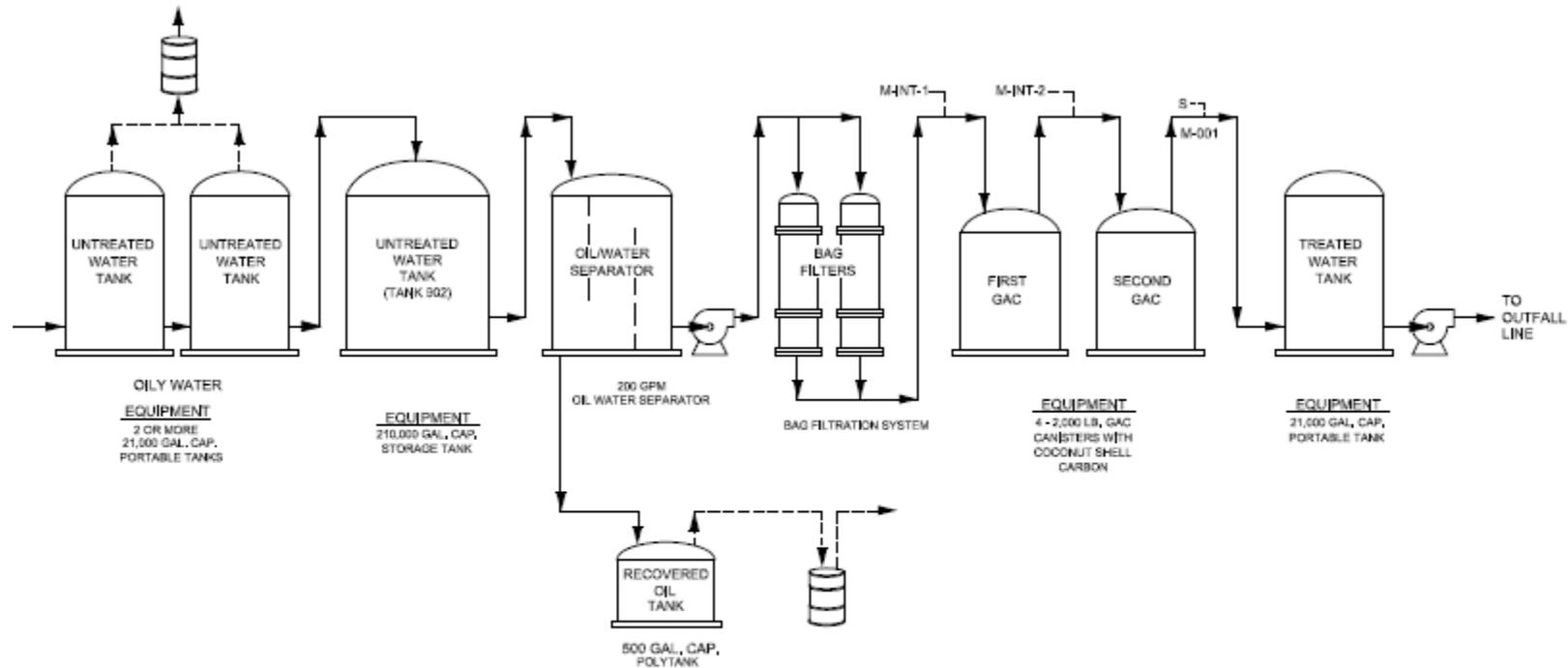
**PROCESS FLOW DIAGRAM - 200 GPM**
