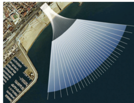
HDD Wells (i.e., Neodren)
