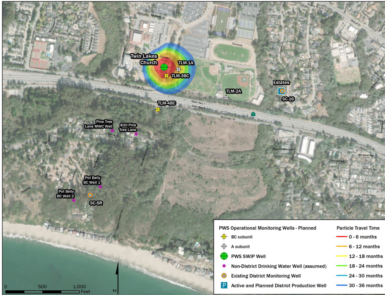
Figure C-6. Map of Twin Lakes Church (TLC) SWIP well, monitoring wells for the Purisima Unit A (TLM-1A and TLM-2A) and Purisima Unit BC (TLM-3BC and TLM-4BC), and modeled subsurface travel times in the Purisima BC Unit from the SWIP well. Figure is from the Final Pure Water Soquel Engineering Report prepared for Soquel Creek Water District, March 2023.
