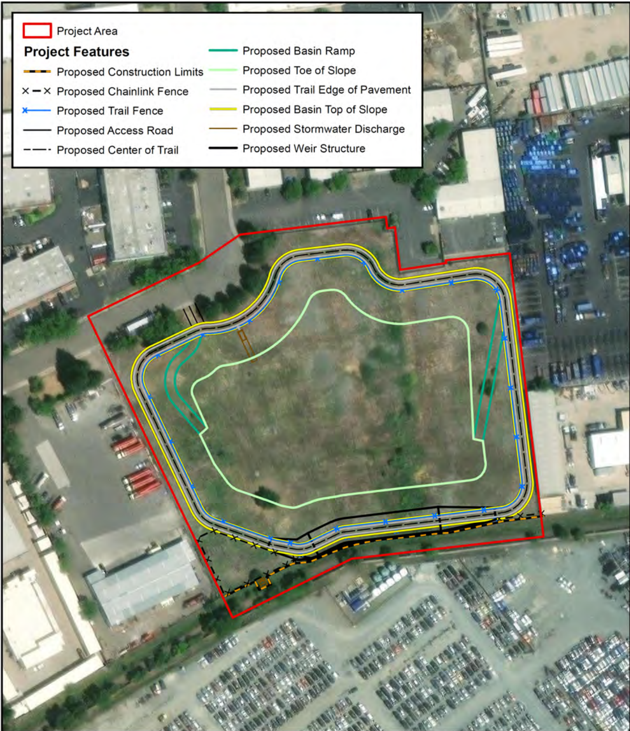
FIGURE 3 PROJECT FEATURES MONIER CIRCLE STORMWATER DETENTION BASIN PROJECT SACRAMENTO COUNTY, CALIFORNIA OCTOBER 2023
