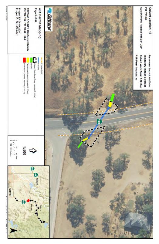
Figure 3: Impacts at Culvert Location 17
