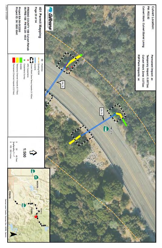
Figure 19: Impacts at Culvert Location 79
