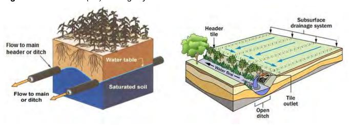
The tile drains are horizontal "pipes", collecting the irrigation water and shallow groundwater to gravity-fed header tile drains that empty into open ditches or sumps that are pumped into a ditch. Tile drains are placed deep enough below the soil surface (about 7 to 8 feet in the GDA) to keep groundwater out of the crop root zone.
