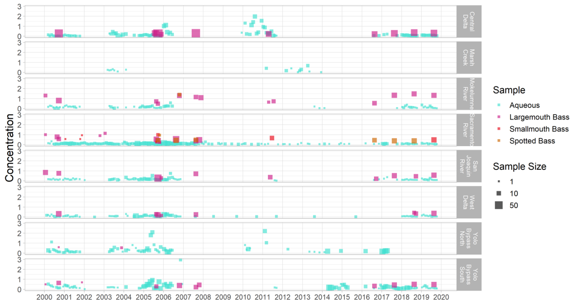
Figure C.1: Monthly Average and Sample Size of Aqueous Methylmercury (ng/L) and Black Bass Mercury (mg/kg) Concentrations in each Subarea
