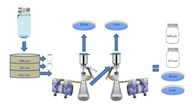
Figure 1: Flow diagram schematic of filtration procedure (Section 11.1).
