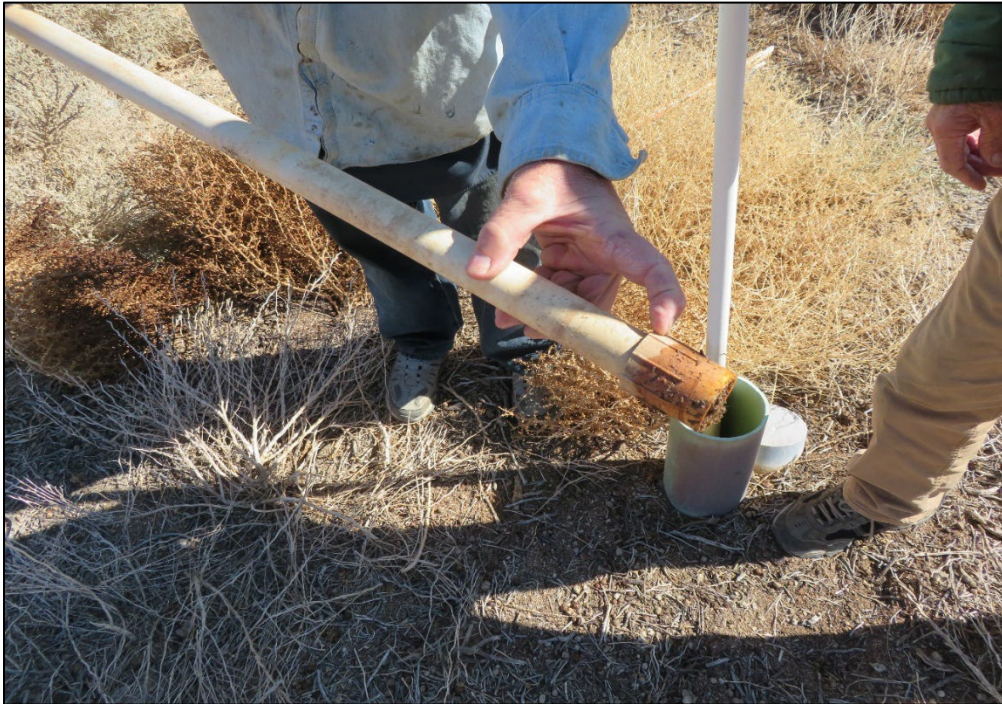
Photo 2.2: The highest water level (approximately 1.5 inches) in the evapotranspiration bed during Water Board visit on February 10, 2025.
