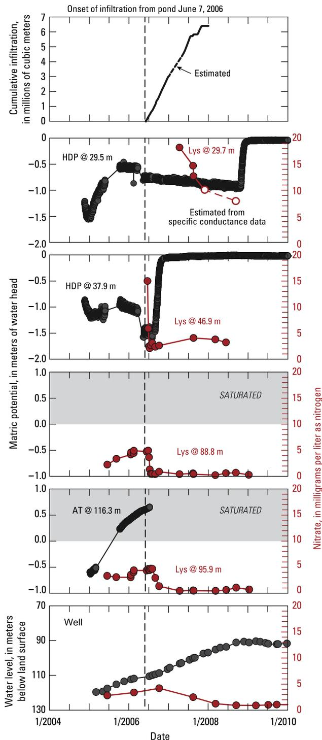
**Fig. 9.** Water level, matric potential, and nitrate concentration data at site YVUZ-1 before and after infiltration from ponds, Warren Groundwater Subbasin, western Mojave Desert, southern California.
