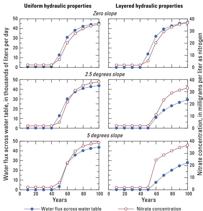
**Fig. 15.** Model simulation results showing water flux across water table and corresponding nitrate concentration for all model configurations for the maximum housing density simulated, 64 0.1 hectare parcels, Warren Groundwater Subbasin, western Mojave Desert, southern California.
