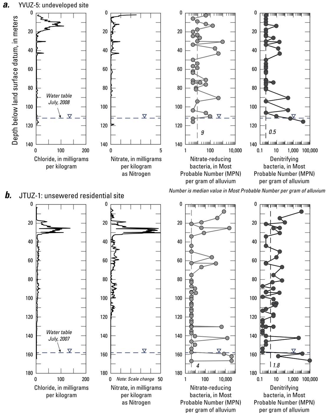
**Fig. 3.** Nitrate, chloride, nitrate reducing bacteria and denitrifying bacteria in unsaturated alluvium at YVUZ-5 and JTUZ-1, Warren Groundwater Subbasin, western Mojave Desert, California, July 2008 and July 2007, respectively.
