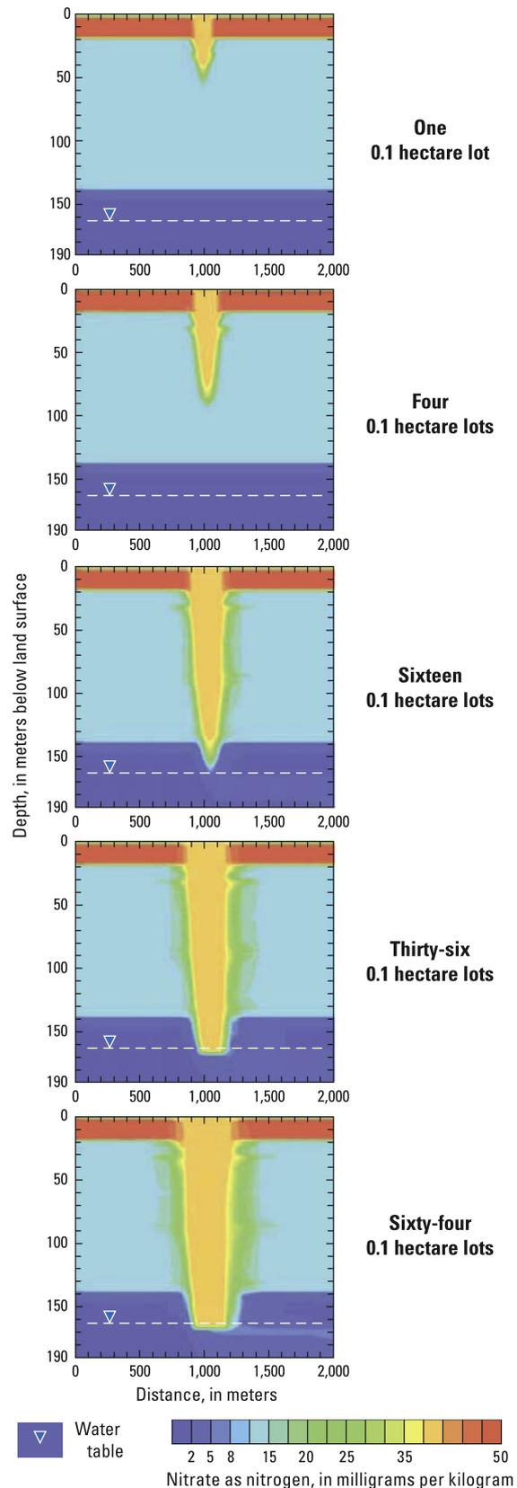
**Fig. 14.** Unsaturated-zone model simulation results showing nitrate concentrations within the unsaturated zone for different housing densities after 100 years for model layers sloping at 2.5°, Warren Groundwater Subbasin, western Mojave Desert, southern California.
