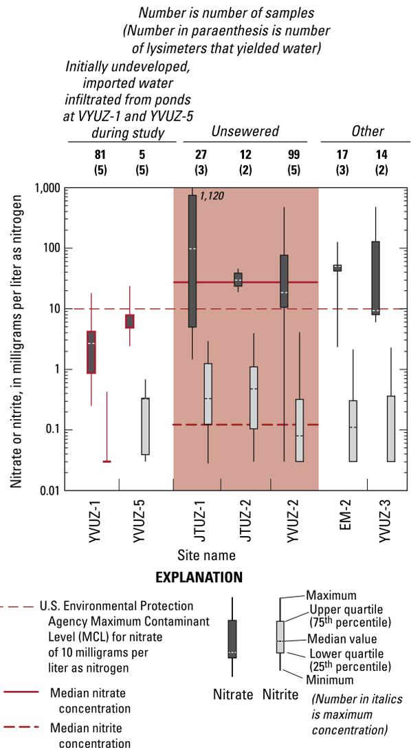
Fig. 7. Nitrate and nitrite concentrations in suction-cup lysimeters within the unsaturated zone at undeveloped, unsewered, and other land uses, Warren, Joshua Tree, and El Mirage Valley Groundwater Subbasins, western Mojave Desert, California, 2005–2014.
