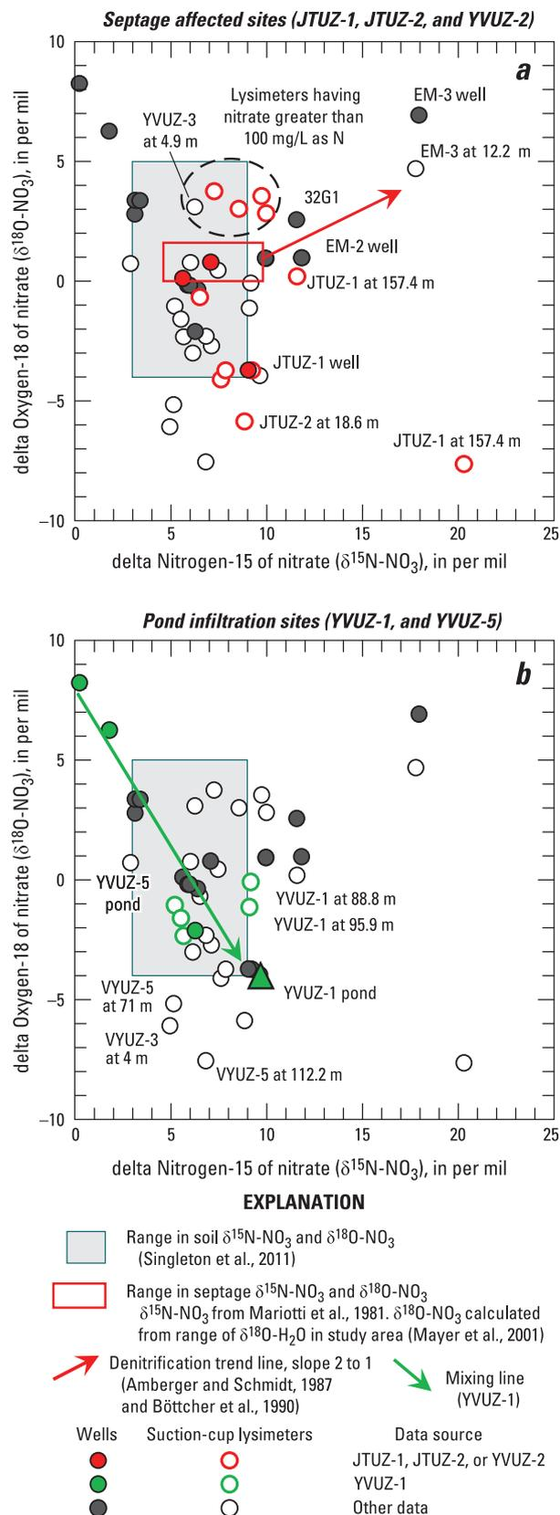
Fig. 12. delta Oxygen-18 of nitrate ( $\delta^{18}\text{O}-\text{NO}_3$ ) as a function of delta nitrogen-15 nitrate ( $\delta^{15}\text{N}-\text{NO}_3$ ) from wells and suction-cup lysimeters at unsewered and dairy wastewater irrigated sites, Warren, Joshua Tree, and El Mirage Valley Groundwater Subbasins, western Mojave Desert, southern California 2006–2009.
