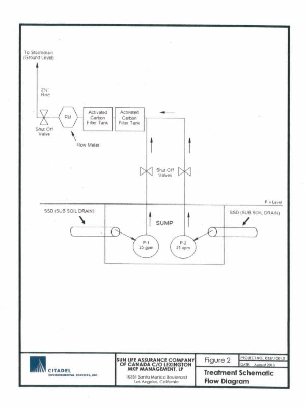
Figure 1. Treatment process flow diagram
