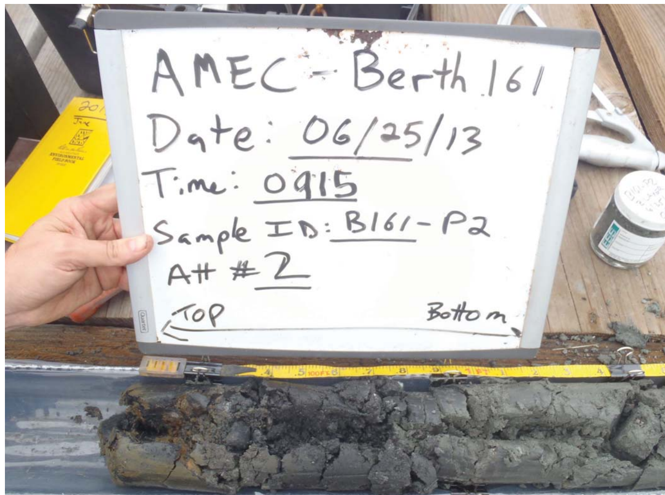
Location: POLA Berth 161 Sample ID: B161-P2 Attempt #: 2 Core Length: 0 - 1.5 ft. Sample Date & Time: 06/25/2013 0915
