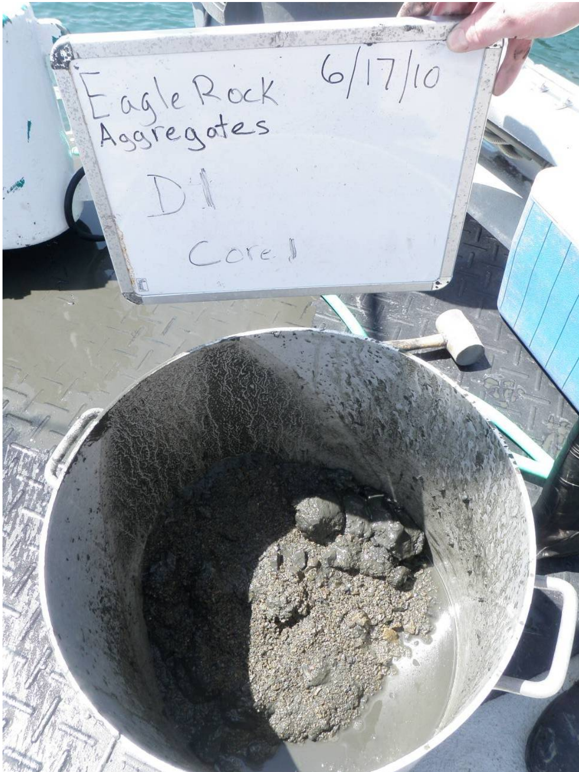
Figure A-1. Core D1 Attempt 1 Following Extrusion of Core into Homogenization Pot.
