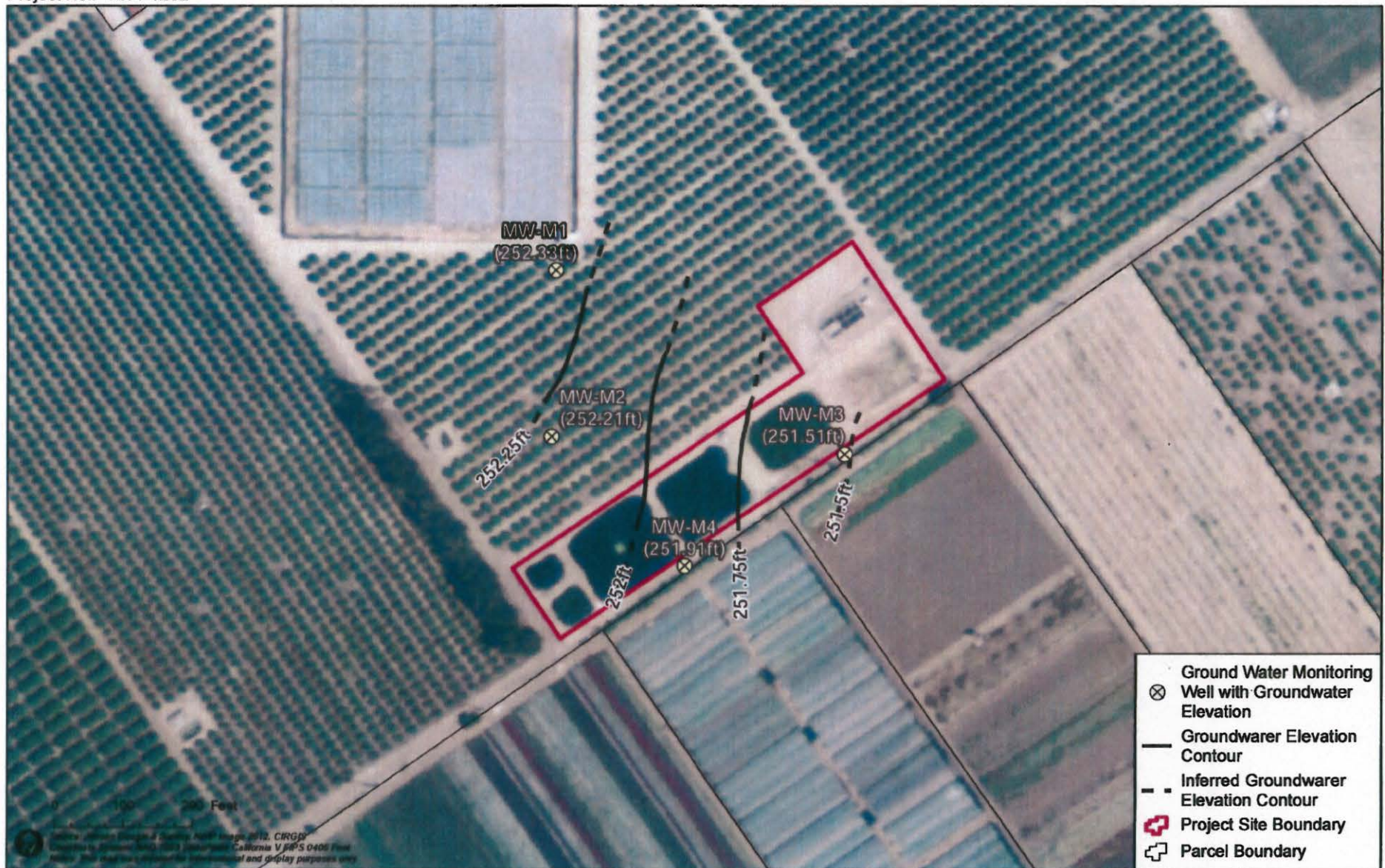
Figure 6. Limoneira WWTP Site Plan and Groundwater Gradient Plan
