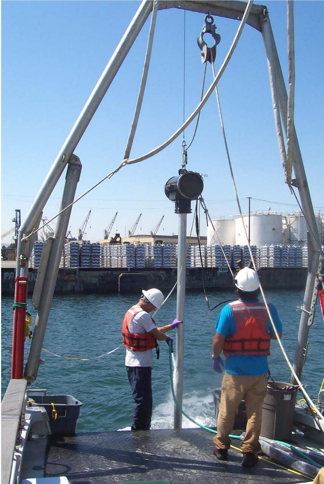
Figure 4. Electric Vibracore Sampler in Long Beach, California
