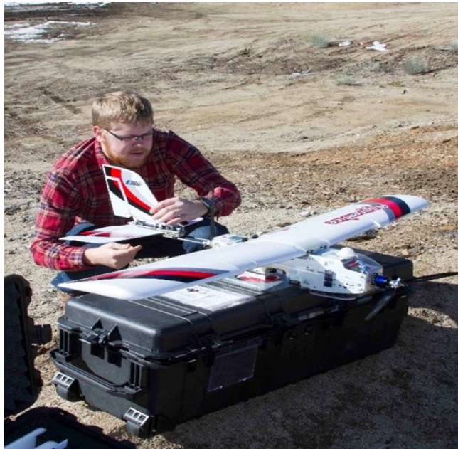
PrecisionHawk engineer conducts a pre-flight test on an unmanned aerial system in the San Bernardino Mountains in January 2016(photo provided by SCCWRP).
