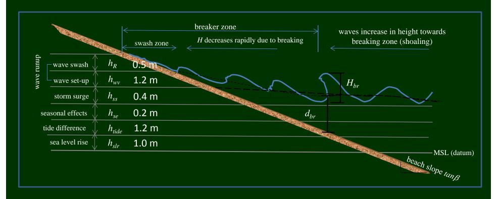
flood level is the combination of rSLR + tides + seasonal effects + storm surge + wave setup + wave runup + fluvial discharge backflow
