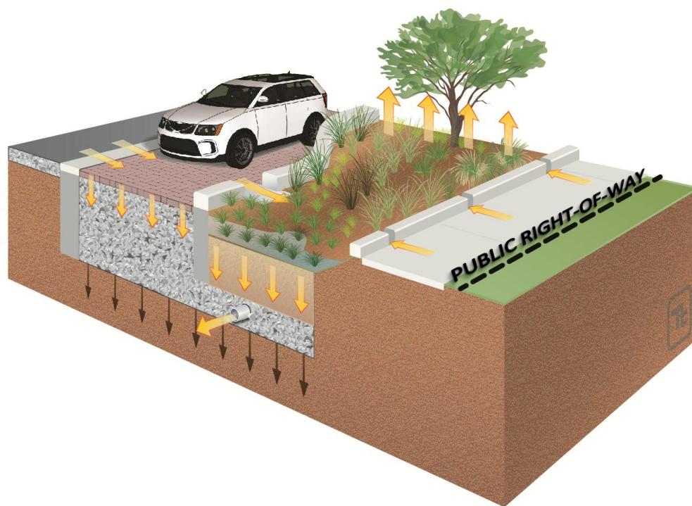
Figure 1-3. Conceptual schematic of ROW BMPs with an underdrain (Arrows indicate water pathways).
