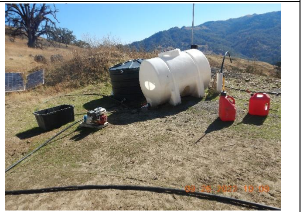
Photo 24 – Improperly stored gasoline tanks, water pump and water storage tanks at WQ9
