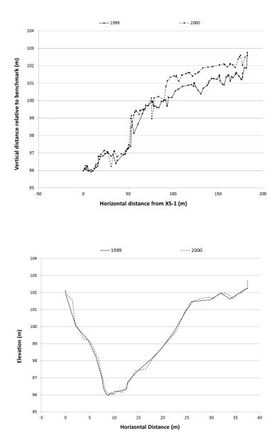
Figure 5. Long profile thalweg survey (above) and cross-section survey (below) data for Stitz Creek ATM-171, 1999-2000
