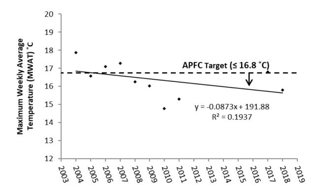
Figure 3. MWAT records at ATM-171 suggest a trend towards the APFC target for stream temperature in Stitz Creek (2004-2018)
