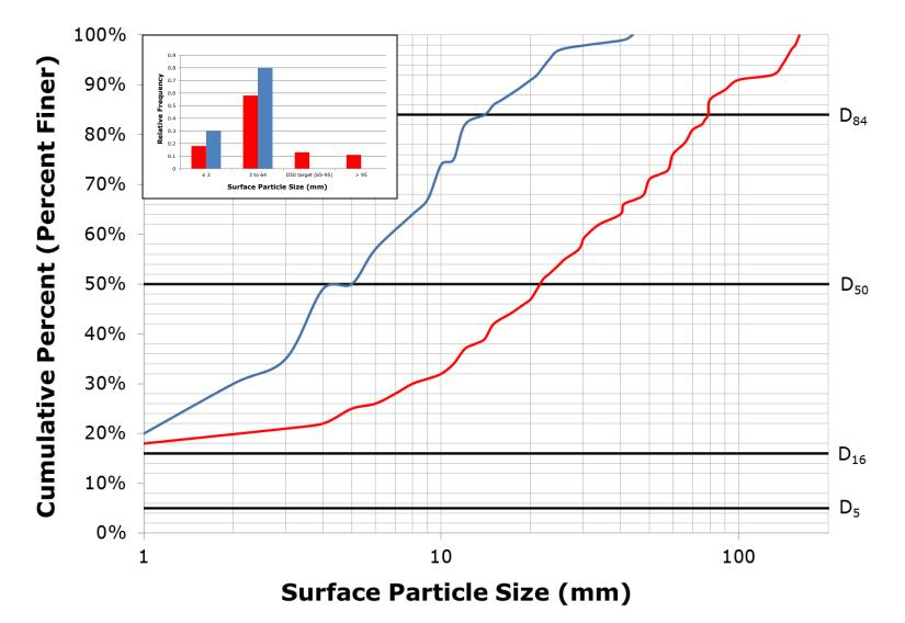
Figure 2. Cumulative percent (percent finer) and corresponding relative frequency distribution (insert) of surface substrate particle sizes\_at ATM-171 (red) and ATM-172 (blue) in Stitz Creek, 2000
