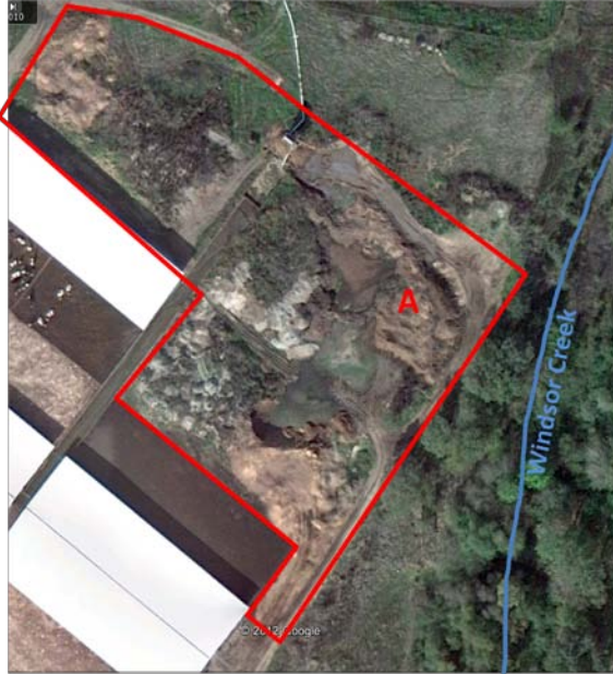
Figure 3-1. Stacked Manure Separated Solids. BMP #3 involves land application of separated manure solids on site. Currently the 12 to 15 foot high piles of manure solids (A) may erode with runoff contributing nutrient loading to the adjacent Windsor Creek. (Manure in the adjacent corral pens is addressed as part of BMP #1.) (Photo Credit Google Earth, taken on October 24, 2009)
