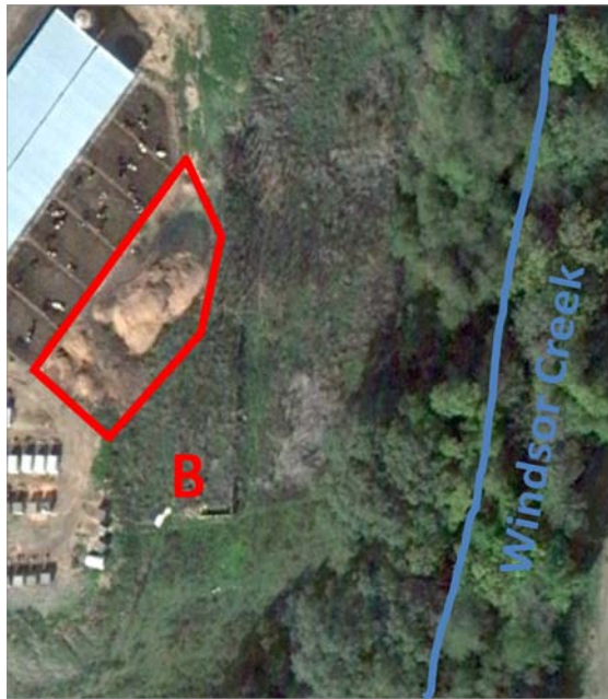
Figure 3-2. Stacked Manure Outside of Calf Barn. BMP #3 involves land application of manure solids on site at agronomic rates. Currently, manure piles dewater in-place contributing to nutrient loading to the adjacent Windsor Creek via runoff. (Photo Credit Google Earth, taken on October 24, 2009)
