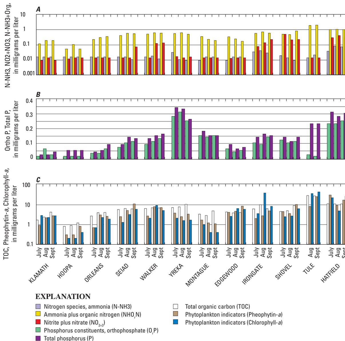
**Figure 10.** Monthly water-quality sampling data for July, August, and September 2002 for six sites on the Klamath River, one site on the Trinity River, three sites on the Shasta River, and two sites on the Lost River in the Lower Klamath River Basin, California. **A.** Nitrogen, **B.** Phosphorus constituents, and **C.** Total organic carbon (TOC), and phytoplankton indicators pheophytin-*a* and chlorophyll-*a*, calculated as concentrations.
