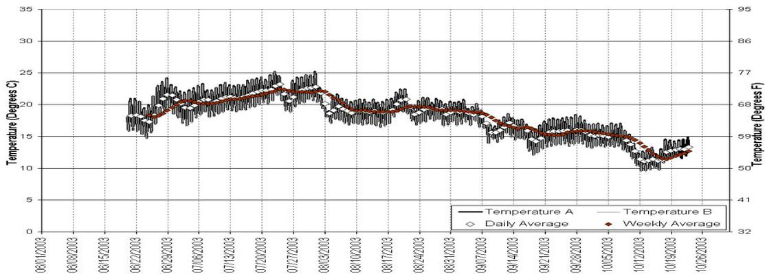
**Figure 47. Continuous Temperature Data - Shasta River @ Freeman Road - Collected by NCRWQCB: 06/01/03 - 10/31/03. (For quality control purposes, two optic StowAway sensors ( A and B ) were deployed at this site).**
