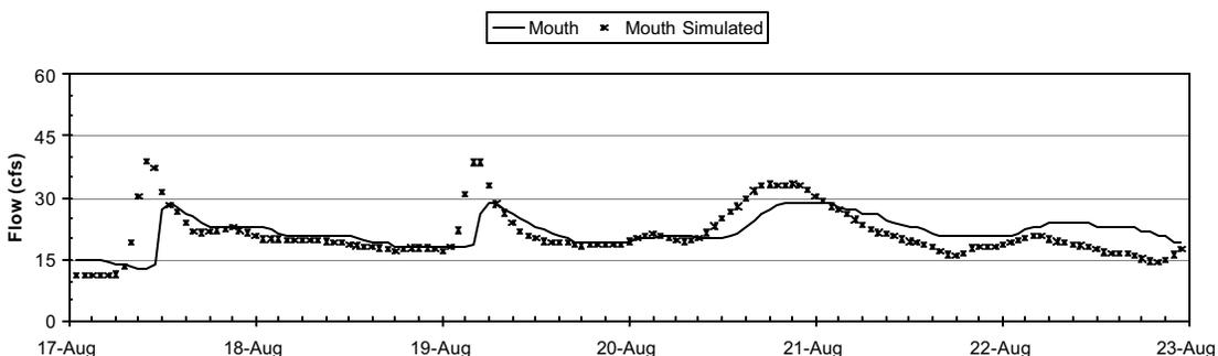
Figure 5-5 Measured vs. simulated flow for Mouth, Aug 17-Aug 23, 2001
