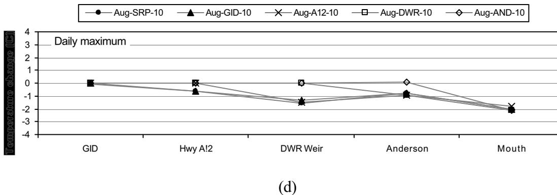
**Figure 5-25 Flow Regime Study results for 10 cfs inflows in August.** Deviations from (a) August base-case condition in (b) daily minima, (c) daily average, and (d) daily maxima of simulated water temperature at GID, Hwy 12, DWR Weir, Anderson Grade Road, and the mouth of the Shasta River.
