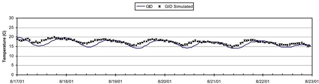
Figure 5-12 Measured vs. simulated temperature for GID, Aug 17-23, 2001
