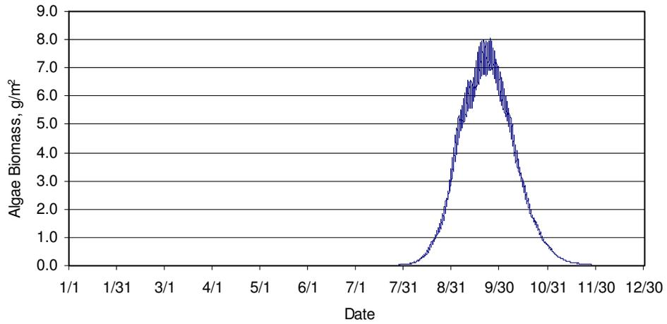
**Figure 31. Algal biomass with TIN concentration equal to 0.02 mg/l, phosphate concentration equal to 0.02 mg/l, and silica concentration equal to 5.0 mg/l**
