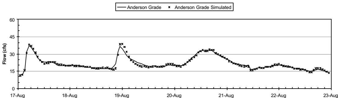
Figure 5-4 Measured vs. simulated flow for Anderson Grade, Aug 17-Aug 23, 2001
