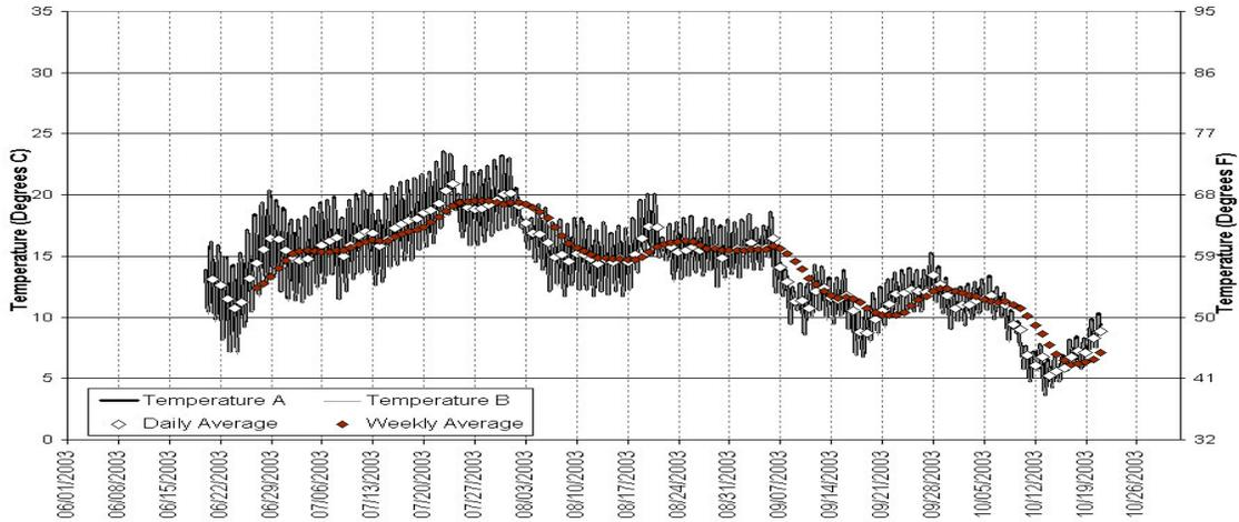
**Figure 50. Continuous Temperature Data – Little Shasta River @ Ball Mountain Road - Collected by NCRWQCB: 06/01/03 - 10/31/03. (For quality control purposes, two optic StowAway sensors ( A and B ) were deployed at this site).**
