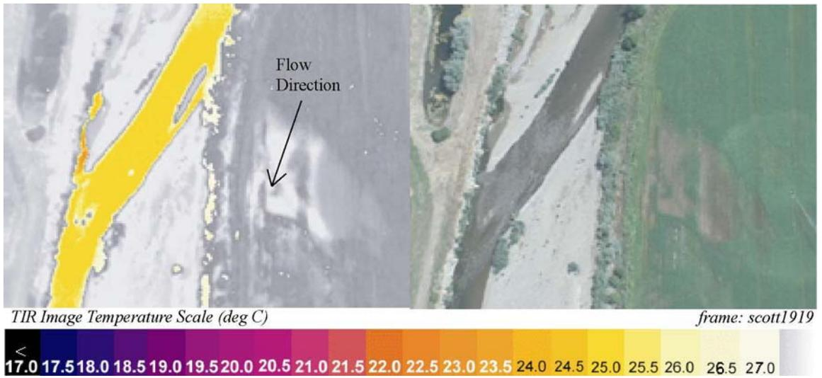
Figure 8 – TIR/color image pair showing an example of a cool water seep detected at river mile 47.2 in the Scott River.
