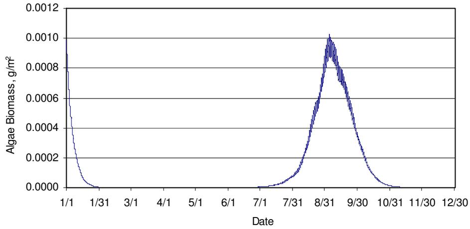
Figure 23. Algal biomass with total inorganic nitrogen concentration equal to 0.014 mg/l
