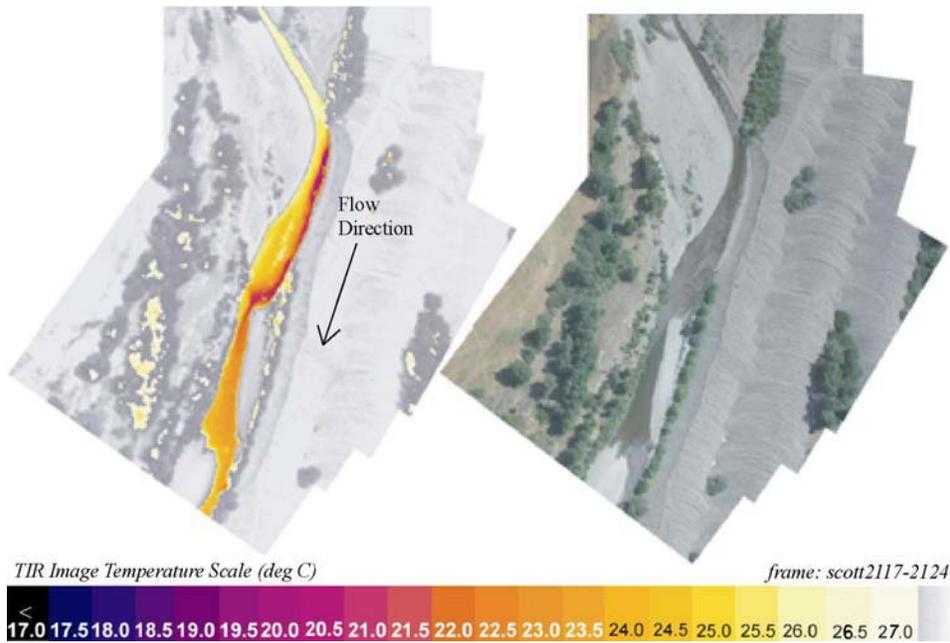
Figure 7 – TIR/color image mosaic showing a sub-surface discharge which appears to emerge from mine tailing along the left bank and decreases water temperatures in the Scott River by  $\approx 3.0^{\circ}\text{C}$  at river mile 52.3.
