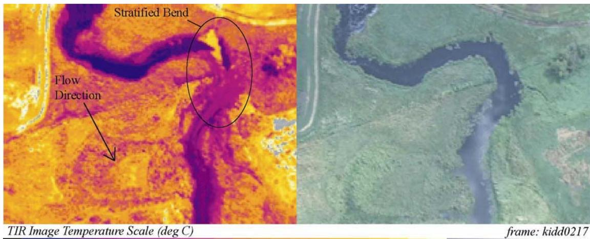
TIR/color video image pair showing a region of Big Slough (25.2°C) at river mile 5.1. The surface temperature pattern around the bend indicates a thermally stratified condition.
