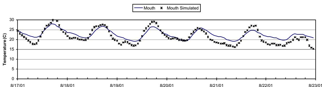
**Figure 5-16 Measured vs. simulated temperature for Mouth, Aug 17-23, 2001**
