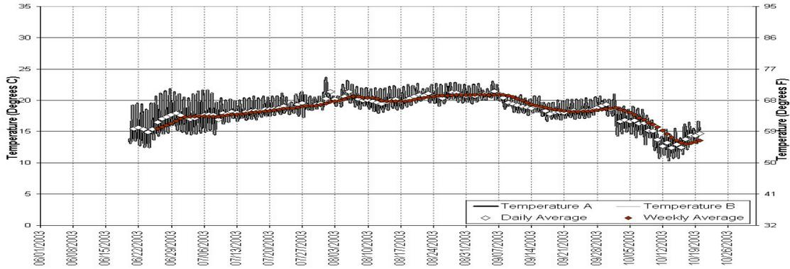
**Figure 45. Continuous Temperature Data - Shasta River @ Riverside Drive - Collected by NCRWQCB: 06/01/03 - 10/31/03. (For quality control purposes, two optic StowAway sensors ( A and B ) were deployed at this site).**
