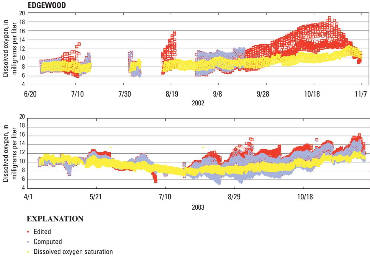
**Figure A2-1.** Measured continuous data of dissolved oxygen with initial edited record, computed record, and saturated values for 2002 and 2003 for USGS sites on the Shasta River, (**A**) EDGEWOOD, (**B**) MONTAGUE, (**C**) HWY3, and (**D**) YREKA.
