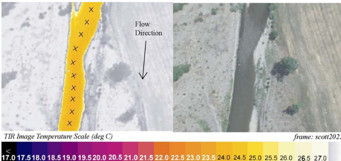
Figure 1 – TIR/color video image pair showing how temperatures are sampled from the TIR images. The black X's on the TIR image show typical sampling locations near the center of the stream channel. The recorded temperature for this image is the median of the sample points.
