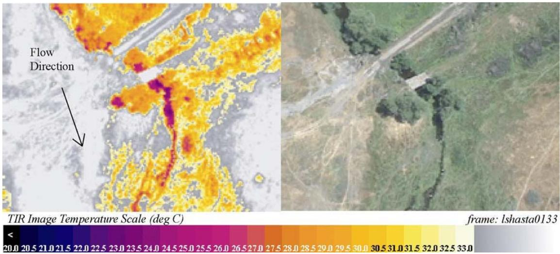
Figure 22 – TIR/color video image showing an example of the localized surface temperature variability on Little Shasta River at river mile 1.3. Median surface temperature upstream of the bridge were 25.7°C while surface temperatures of 23.3°C were recorded in the shaded area downstream of the bridge. The difference suggest differential surface heating in the shaded areas or thermal stratification upstream of the bridge.
