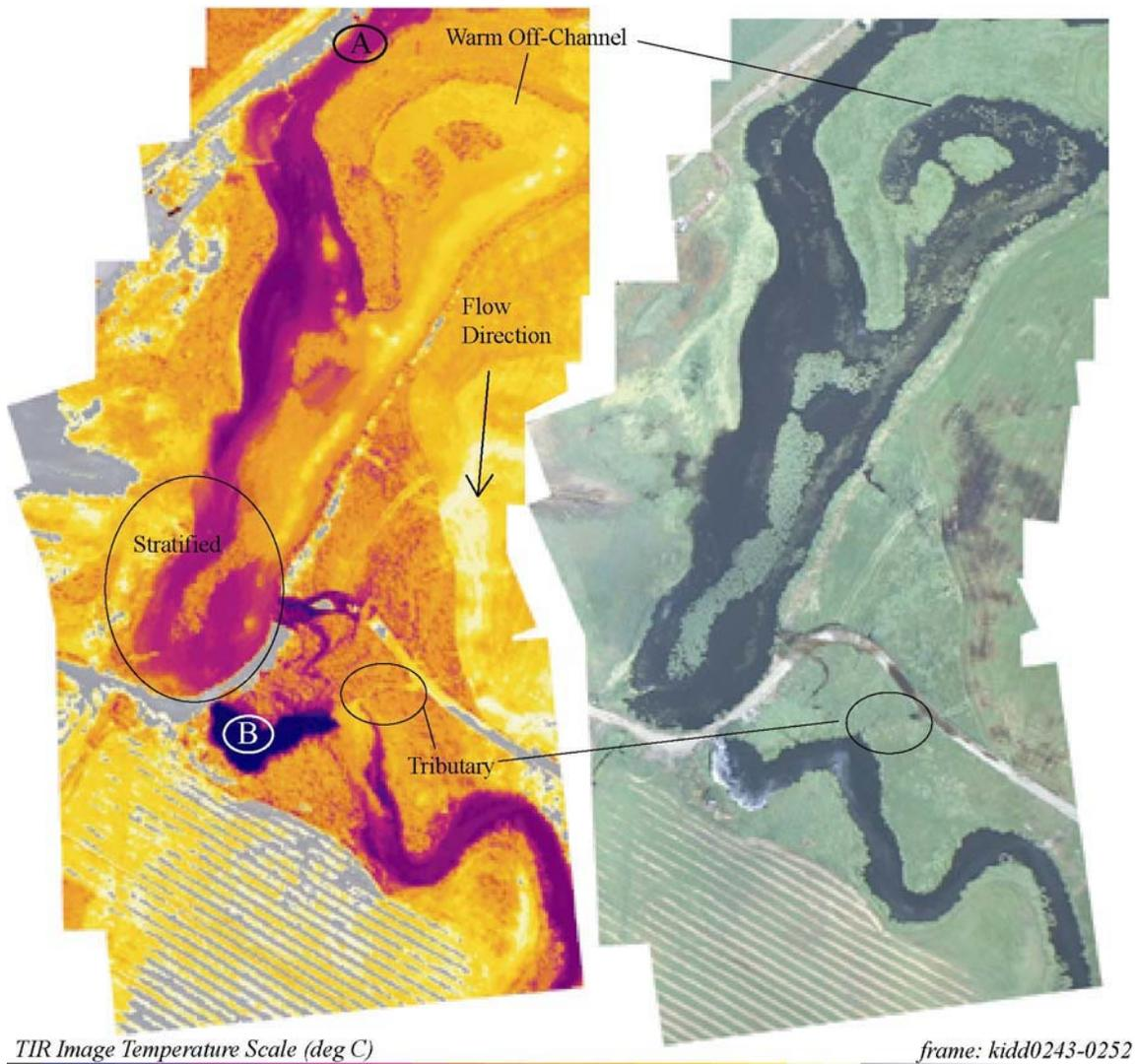
TIR/color video image pair showing a stratified stretch of Big Slough with an unnamed warm tributary (32.0°C) on the left bank, in the bottom half of the image. The temperature at point A is 25.4°C while the temperature directly downstream of the bridge (B) is 23.9°C (river mile 6.0).
