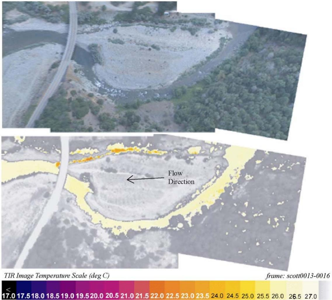
TIR/color video image pair showing a spring (22.1°C) in the side channel on the right bank of the Scott River (25.9°C) at river mile 0.2.
