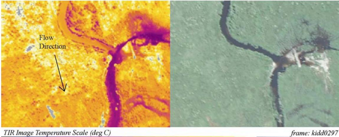
TIR/color video image pair showing a transition in Big Slough from a stratified state to a mixed condition moving downstream at river mile 7.5.
