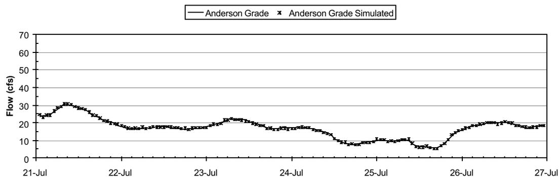
Figure 5-9 Measured vs. simulated flow for Anderson Grade, July 21-July 27, 2001
