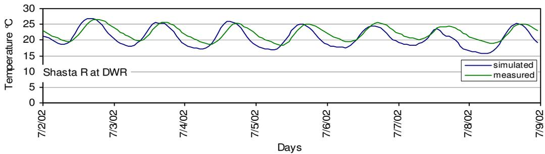
**Figure 33. Temperature DWR Weir for 7/02/2002 – 7/08/2002**
