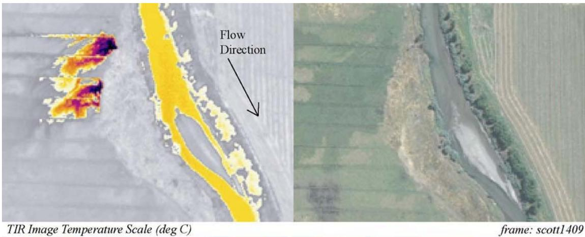
TIR/color video image pair showing a thermal signature in a field near right bank of the Scott River (24.5 °C) at river mile 36.5. This thermal signature is presumed due to transpiring vegetation from irrigation or recent rain.
