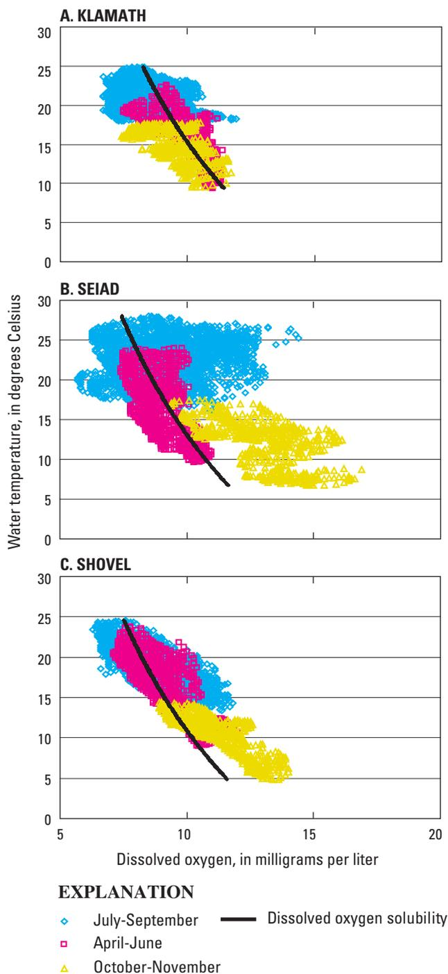
**Figure 6.** Relation between water temperature and dissolved oxygen (DO) for continuous water-quality monitoring stations at in the Lower Klamath River Basin, California, 2002 and 2003. **A**, KLAMATH; **B**, SEIAD; and **C**, SHOVEL.
