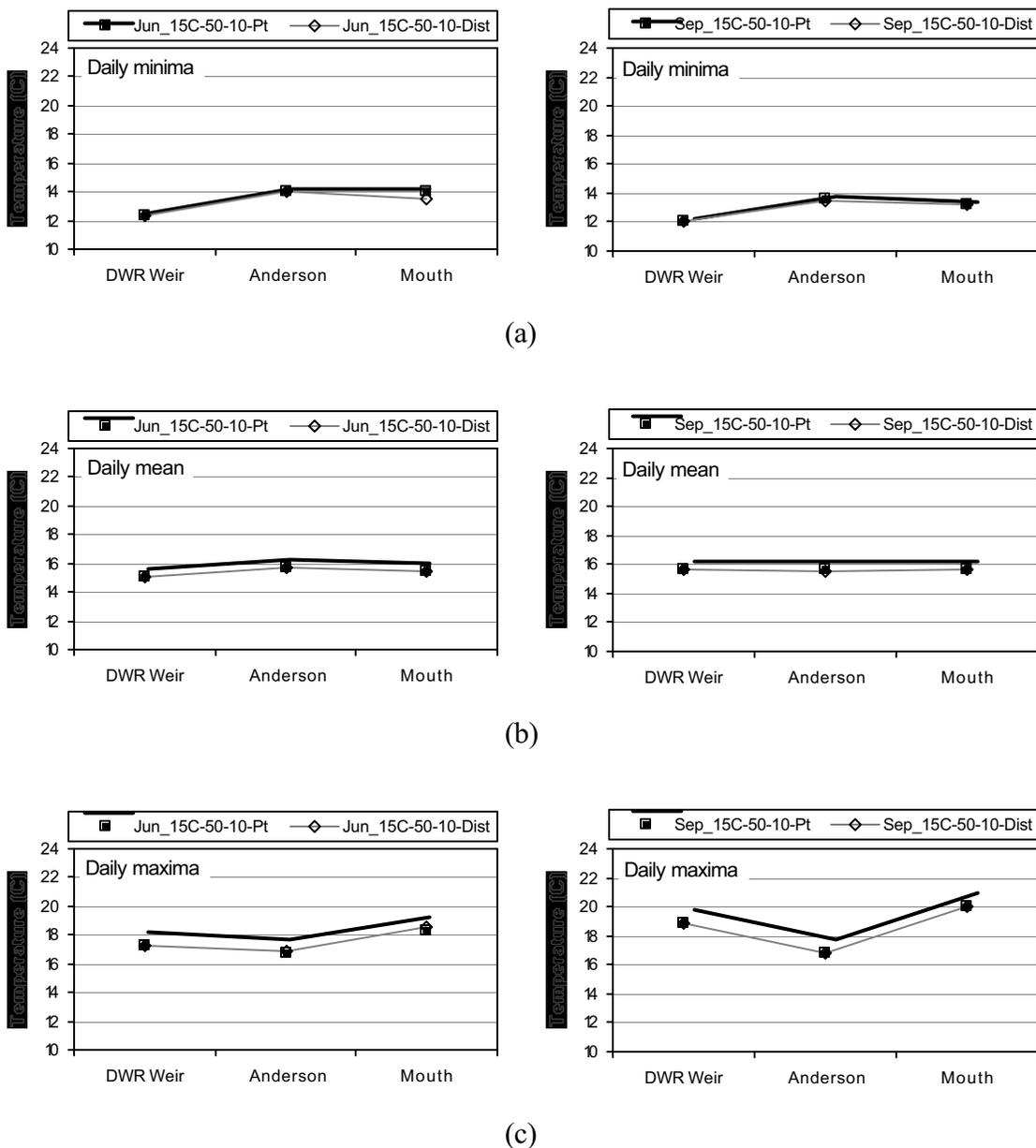
**Figure 5-34 Tailwater Return Study 15°C-50-10 results for June and September.** Upstream boundary condition of 15°C and 50 cfs at SRP, tailwater return flow of 10 cfs. Simulated (a) daily minimum, (b) daily average, and (c) daily maximum water temperature at DWR Weir, Anderson Grade Road, and the mouth of the Shasta River comparing point and distributed discharge of tailwater. Simulations designated by “month\_upstream water temperature-upstream inflow-tailwater flow” (e.g. Sep\_15C-50-10).
