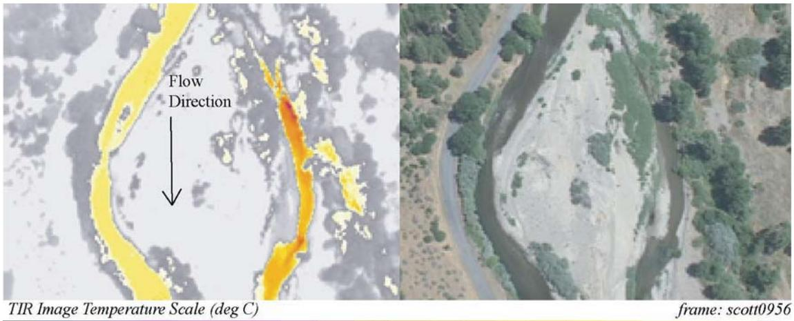
TIR/color video image pair showing a spring/seep emerging from within the left bank channel of the Scott River (25.3 °C) at river mile 24.5.
