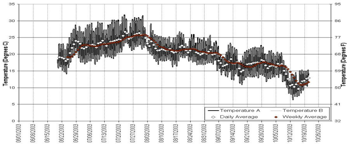
**Figure 51. Continuous Temperature Data – Little Shasta River near Mouth - Collected by NCRWQCB: 06/01/03 - 10/31/03. (For quality control purposes, two optic StowAway sensors ( A and B ) were deployed at this site).**
