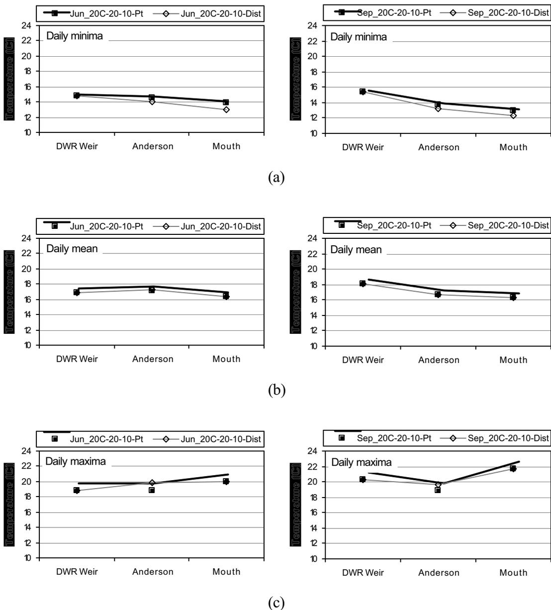
**Figure 5-36 Tailwater Return Study 20°C-20-10 results for June and September.** Upstream boundary condition of 20°C and 20 cfs at SRP, tailwater return flow of 5 cfs. Simulated (a) daily minimum, (b) daily average, and (c) daily maximum water temperature at DWR Weir, Anderson Grade Road, and the mouth of the Shasta River comparing point and distributed discharge of tailwater. Simulations designated by “month\_upstream water temperature-upstream inflow-tailwater flow” (e.g. Sep\_20C-20-10).
