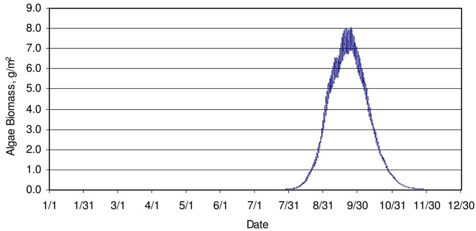
**Figure 16. Algal biomass with nitrogen half saturation coefficient equal to 0.14 mg/l**
