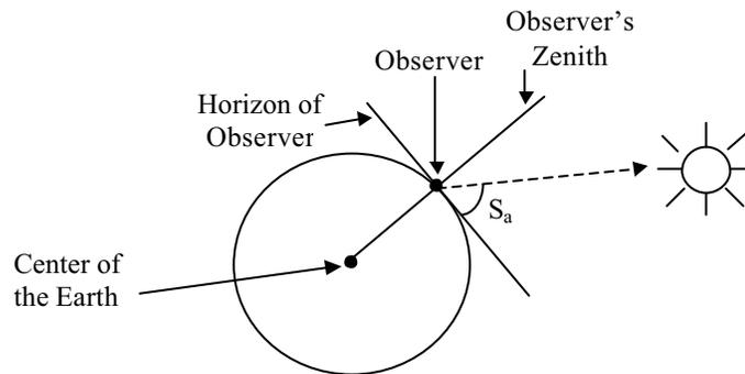
**Figure 2-1 Diagram of the solar altitude**
