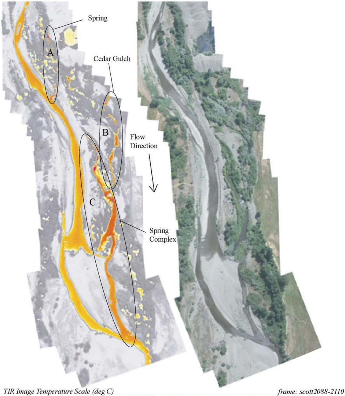
TIR/color video image pair showing a spring complex (C) (22.5 °C) on the left bank of the Scott River (24.1 °C). Cedar Gulch (B) can be seen on the left bank of the Scott River; however, because it's confluence with the Scott cannot be determined, it was not sampled. There is also a spring (A) (20.0 °C) on the left bank of the Scott upstream of Cedar Gulch, at river mile 52.0.
