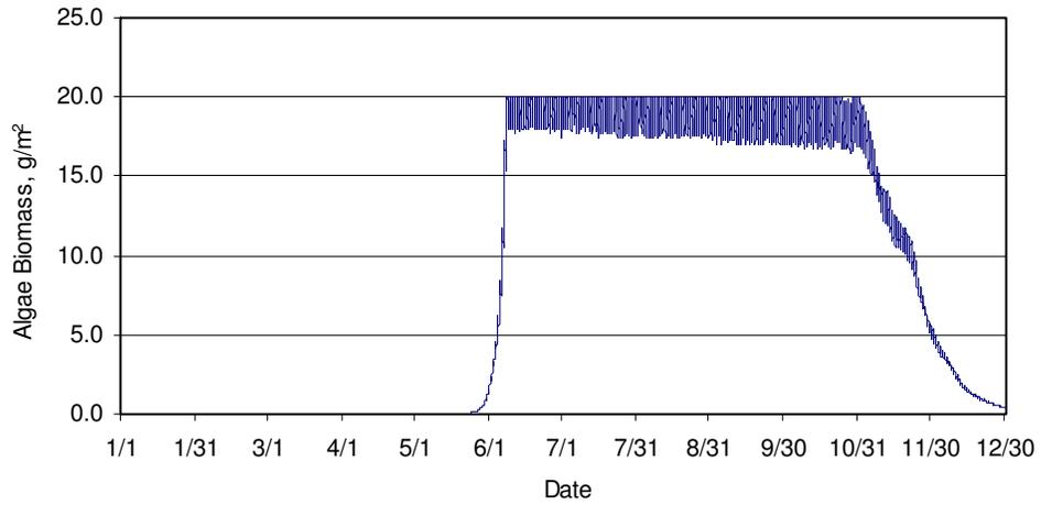
**Figure 19. Algal biomass with silica half saturation coefficient equal to 0.003 mg/l**
