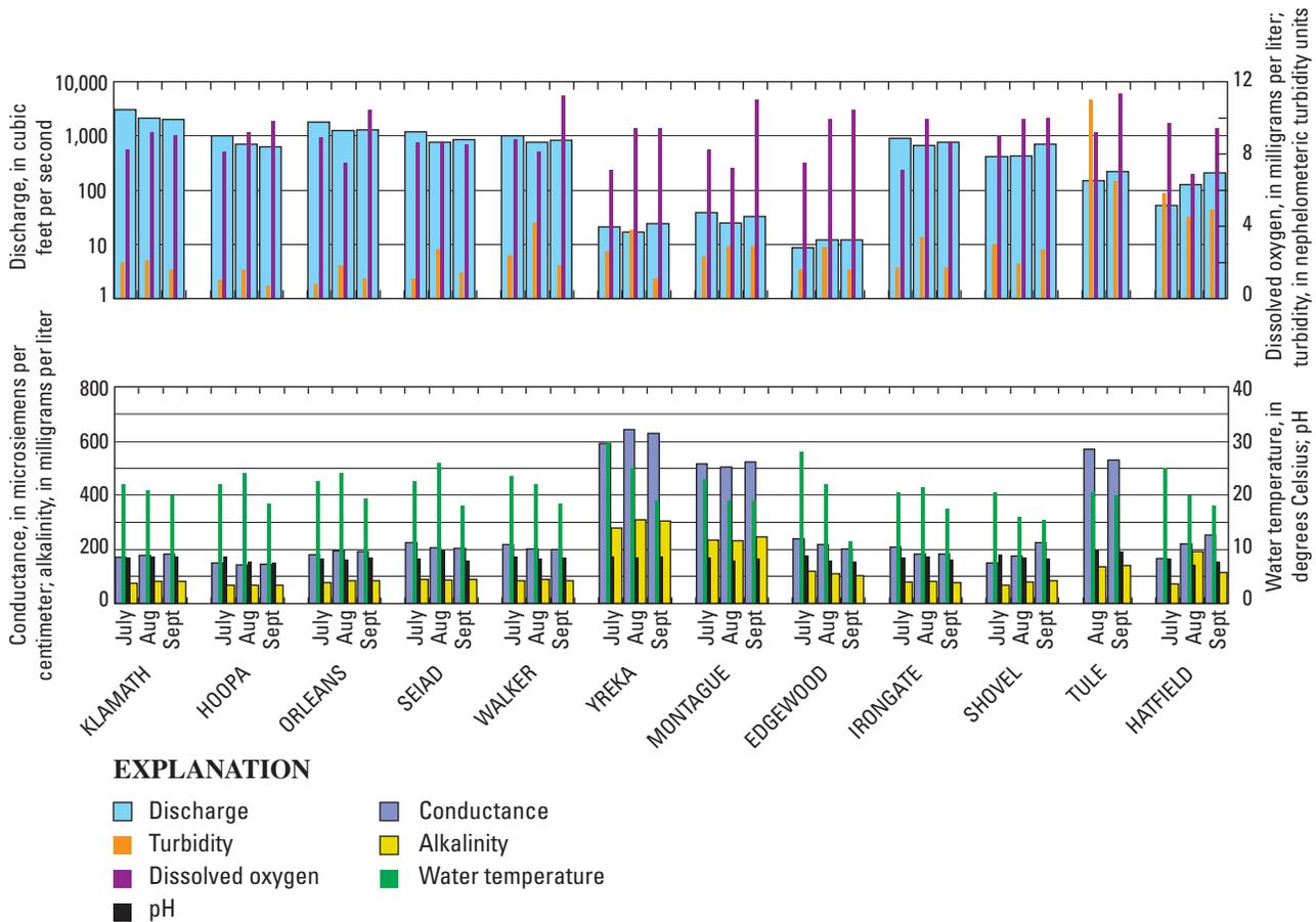
**Figure 9.** Monthly water-quality sampling data for July, August, and September 2002 for six sites on the Klamath River, one site on the Trinity River, three sites on the Shasta River, and two sites on the Lost River in the Lower Klamath River Basin, California. **A.** Instantaneous discharge, dissolved oxygen (DO), and turbidity, and **B.** Specific conductance, alkalinity, water temperature, and pH.
