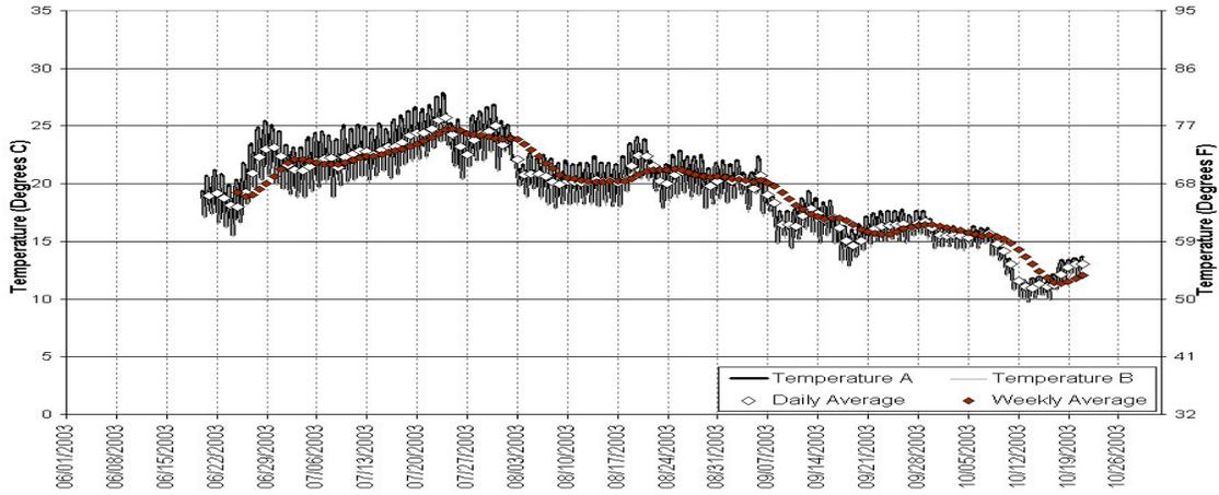
**Figure 48. Continuous Temperature Data - Shasta River @ Yreka-Ager Road - Collected by NCRWQCB: 06/01/03 - 10/31/03. (For quality control purposes, two optic StowAway sensors ( A and B ) were deployed at this site).**
