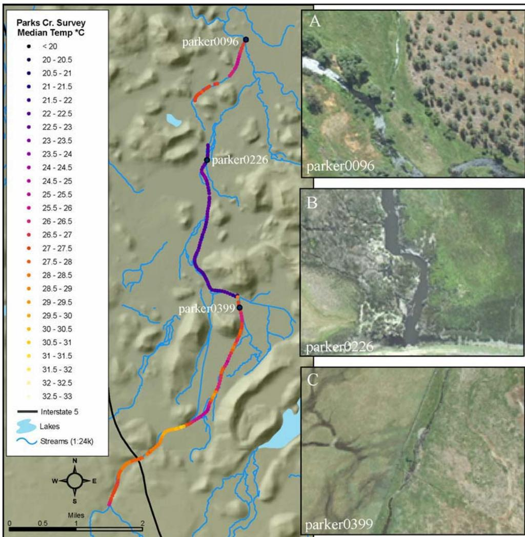
Figure 23 – A series of three true color video images illustrating changes in channel characteristics over the 10-mile survey length of Parks Creek. Image A shows the mouth of Parks Creek, illustrating the narrow channel width compared with the Shasta River. Image B shows Parks Creek at river mile 2.6, with a wider channel than is seen upstream at river mile 5.7 (Image C).
