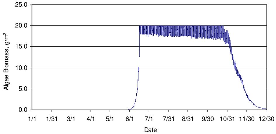
**Figure 27. Algal biomass with phosphate concentration equal to 0.02 mg/l**
