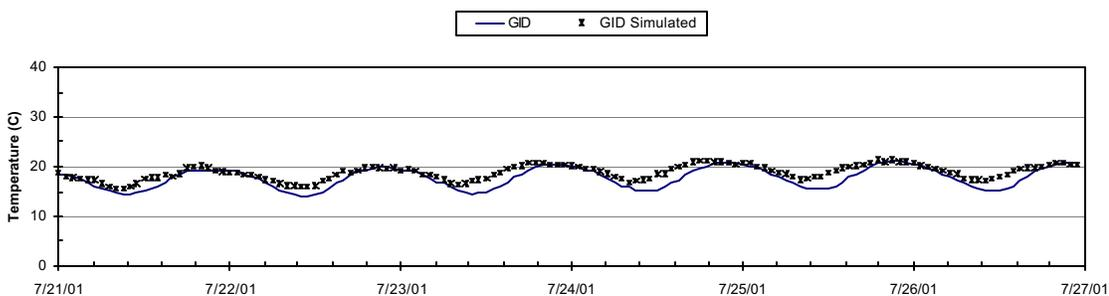
**Figure 5-18 Measured vs. simulated temperature for GID, July 21-27, 2001**
