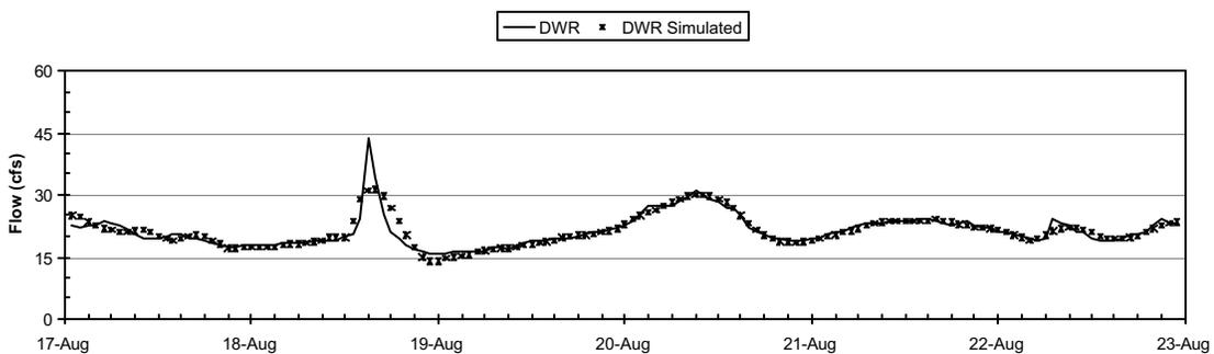
Figure 5-3 Measured vs. simulated flow for DWR Weir, Aug 17-Aug 23, 2001
