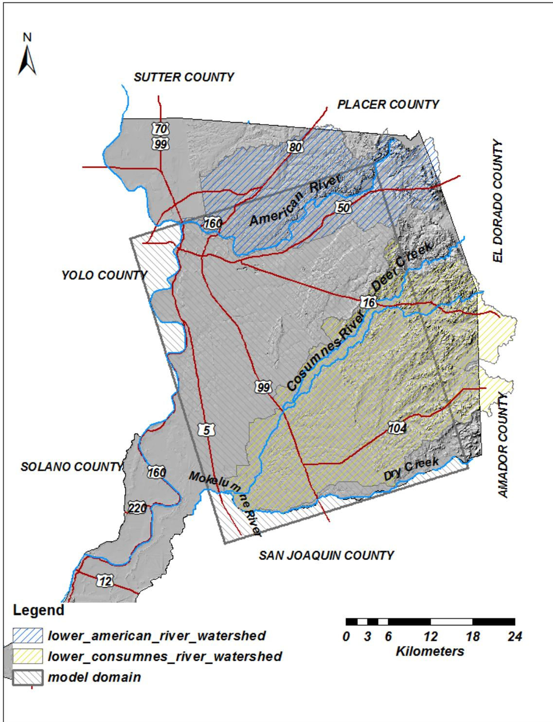
Figure 2.1 Study area major hydrologic features and numeric model domain.
