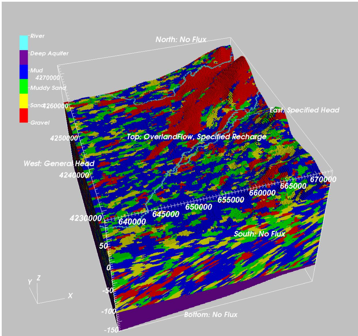
**Figure 3.7 Numerical model domain and boundary conditions (the bottom purple segment represents added layers for representing deeper aquifer system. Coordinates are in WGS84-UTM10N coordinate system).**
