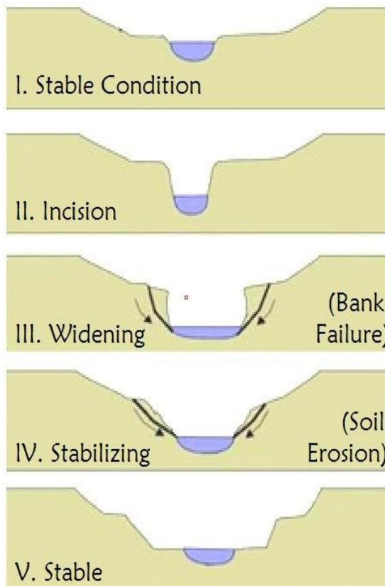
Figure 1. Graphic depicting a river cross-section as it succumbs to incision and subsequently adapts. (2003, USGS)
