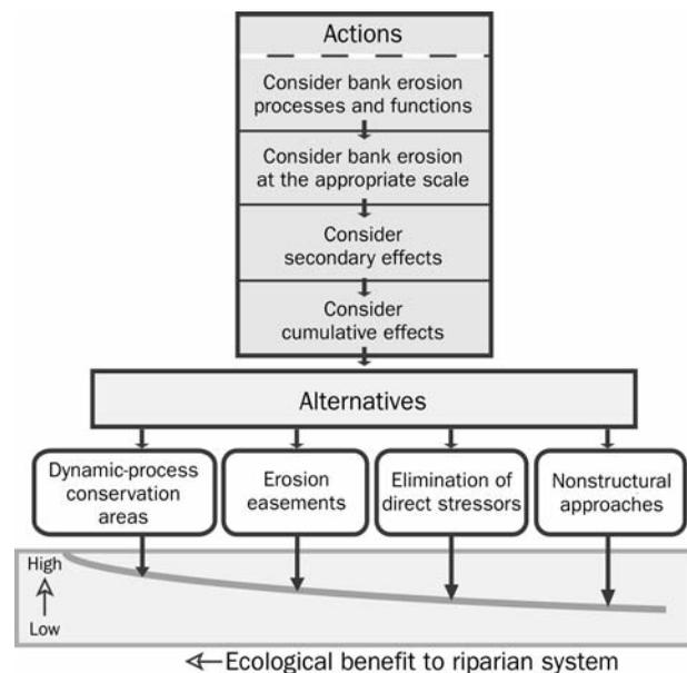
**Figure 5.** Framework for alternatives to channel bank infrastructure. *Dynamic-process conservation areas* protect the linkage between river channels and adjacent landscapes, and provide the highest ecological benefit to riparian ecosystems. The other alternatives provide ecological benefits to the degree that they accommodate the geomorphic processes that sustain them.
