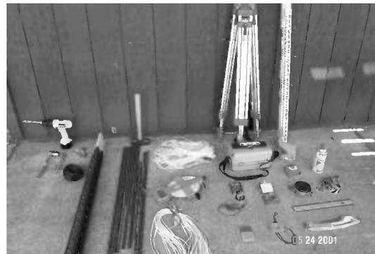
**Figure 10:** Surveying Equipment
