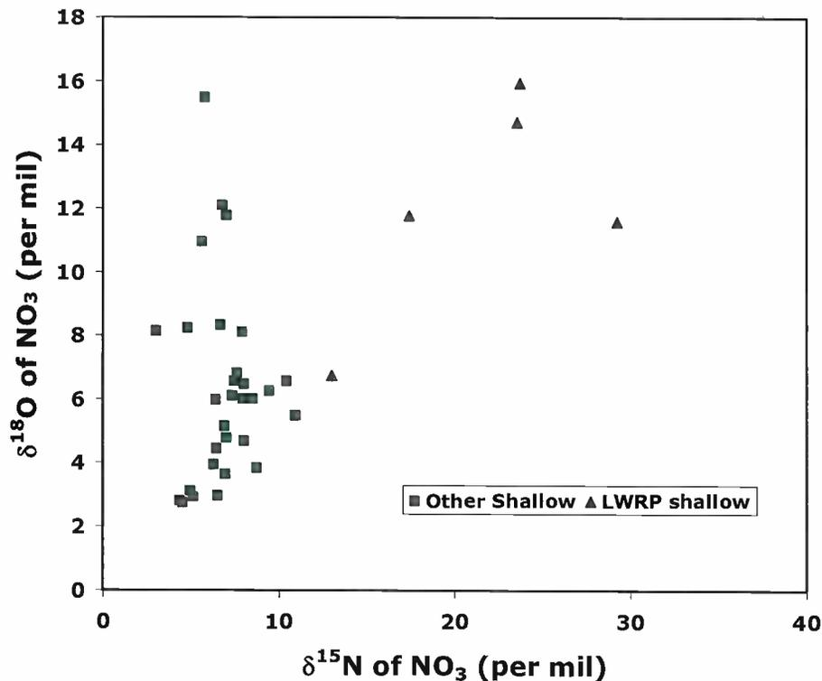
**Figure 26.** Shallow wells whose recharge source is treated wastewater from LWRP have isotopic signatures of nitrate that are distinct from other wells and indicate isotopic fractionation mediated by denitrification.
