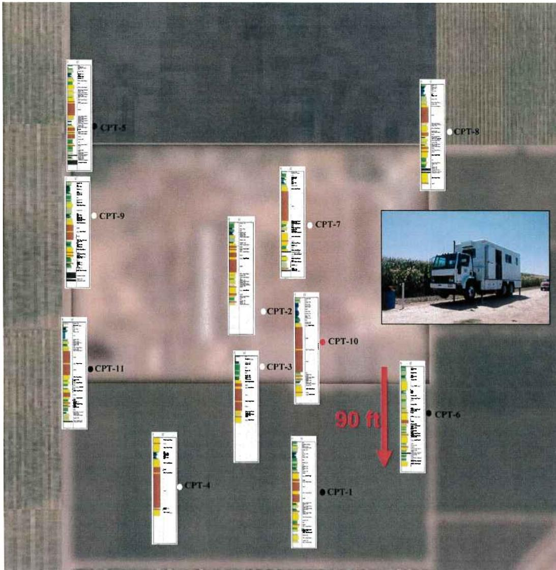
**Figure 3. KCD1 field site with CPT/DP locations.**
