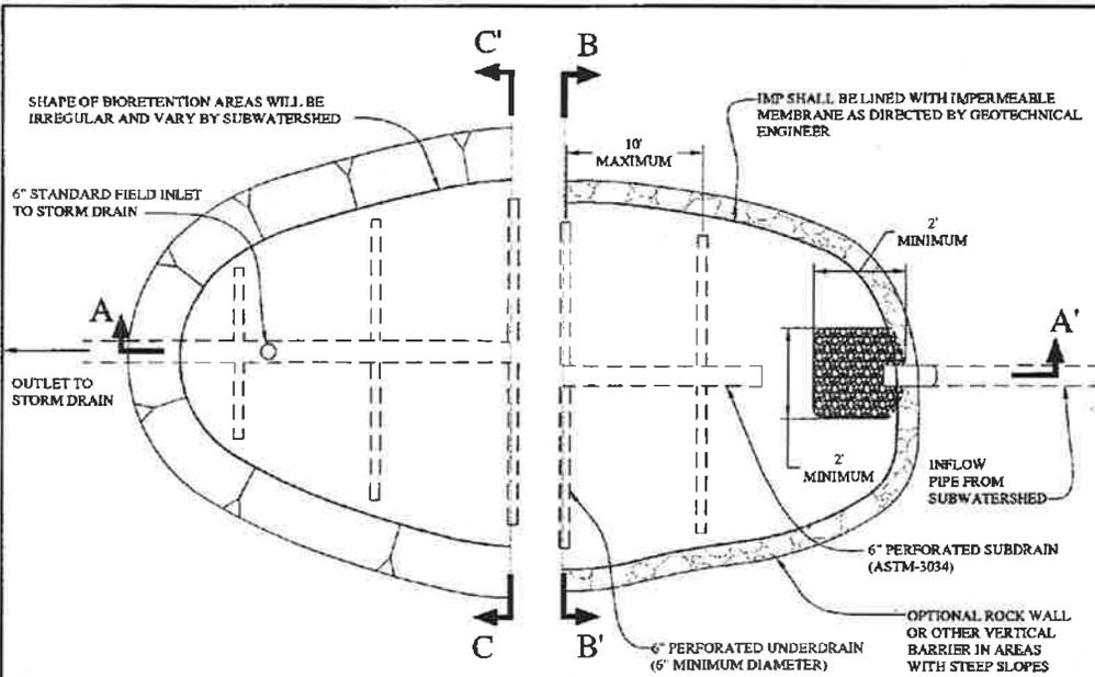
**TYPICAL BIORETENTION AREA WITH 3:1 SIDE SLOPES - PLAN VIEW**
