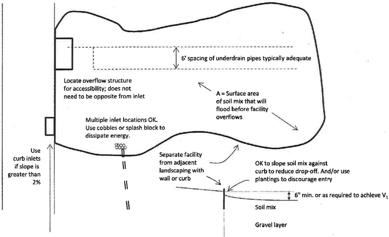
Note: Call out elevations of curb, pavement, inlet, top of soil layer (TSL), bottom of soil layer (BSL), and bottom of gravel layer (BGL) at all inlets and outlets and at key points along edge of facility.
