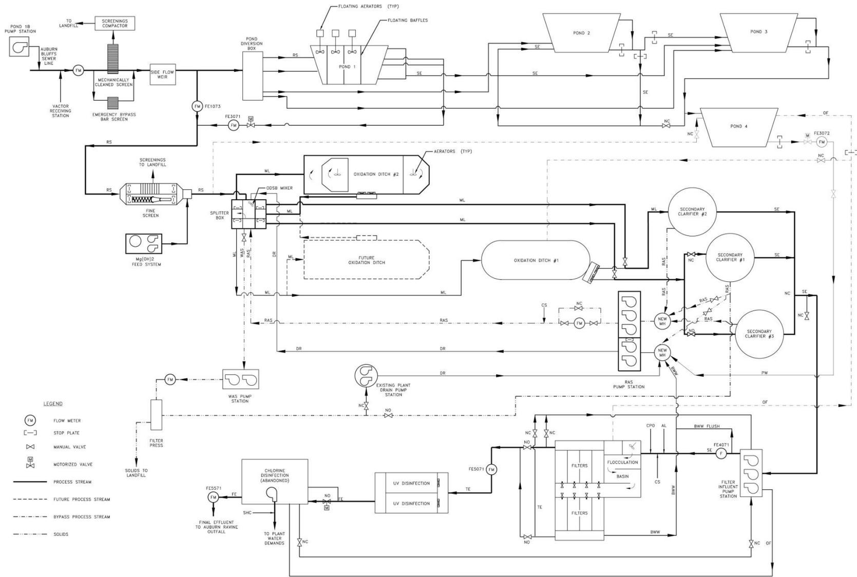
**Process Flow Diagram for the Proposed City of Auburn WWTU Upgrades**
