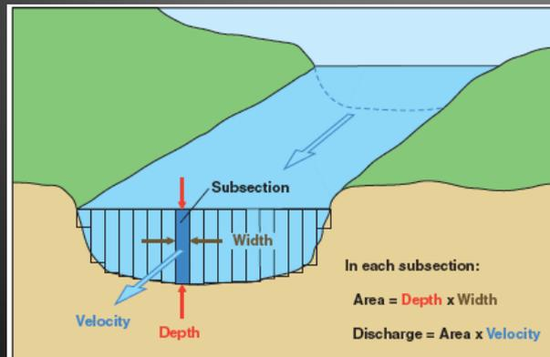
Current-meter discharge measurements are made by determining the discharge in each subsection of a channel cross section and summing the subsection discharges to obtain a total discharge.
