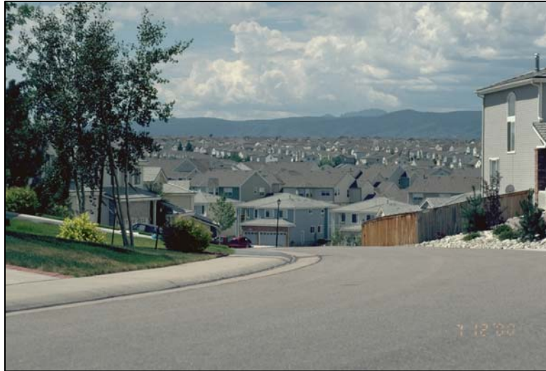
Photograph RO-2—Urbanization (impervious area) increases runoff volumes, peak discharges, frequency of runoff, and receiving stream degradation.
