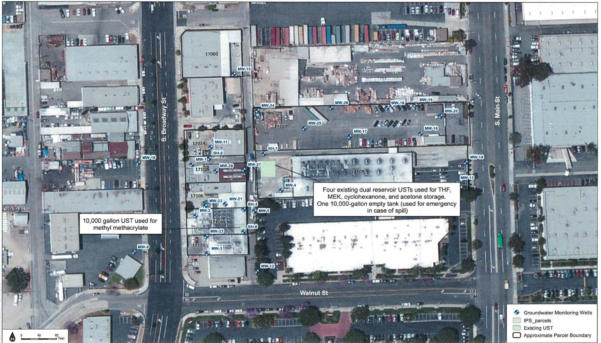
FIGURE 1 Site Layout with Monitoring Wells and USTs
